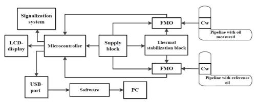
Fig. 3. Block diagram of the system for measuring and controlling humidity in crude oil and petroleum products [19].
