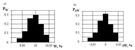
Fig. 6. Frequency histograms: a) probabilities of values of the Turkmen Blend crude oil humidity, b) probabilities of measurement error values.
