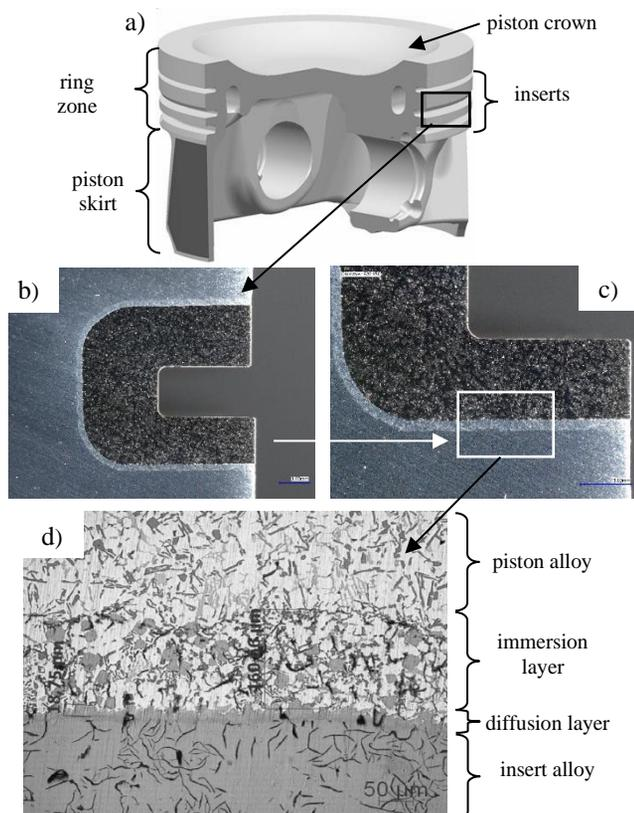
Fig. 2. Gasoline piston a); macrostructure of the insert-piston contact area b, c); microstructure of the insert-piston junction d)
