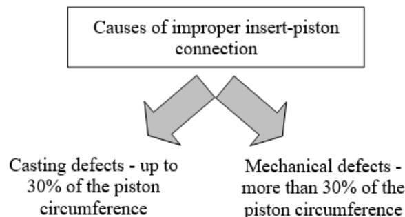
Fig. 3. Classification of the causes of the improper connection between the cast iron ring insert and the piston body.
