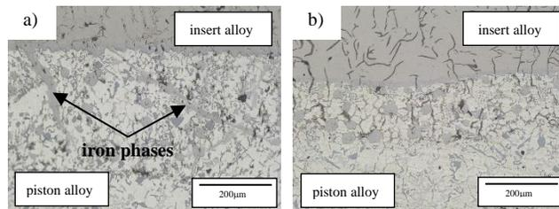
Fig. 6. Microstructure of the insert-piston joint: above 0.35 wt% Fe a); up to 0.35 wt% Fe b)
