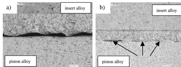
Fig. 7. Microstructure of the improper liner-piston connection: no immersion layer a); so-called oxide "film" (arrows) b)
