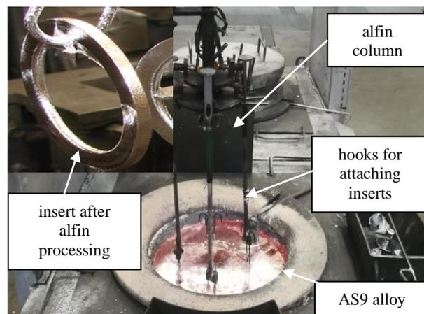
Fig. 1. Industrial stand for ring inserts alfin processing
