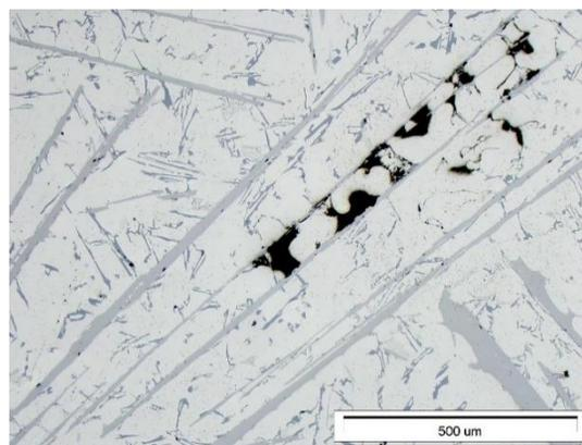
Fig. 8. Long (more than about 500  $\mu\text{m}$ )  $\beta$ -Al<sub>5</sub>FeSi phase precipitates along with visible shrinkage porosity
