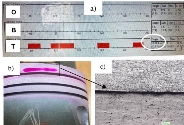
Fig. 5. An example of a casting defect at the insert-piston interface: screenshot from Harrandt systems a); location of the defect b); microstructure within the localized defect c)
