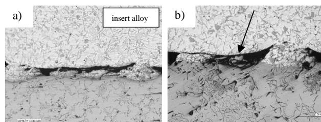
Fig. 11. Microstructure of improper insert-piston connection a), visible dirt and inclusions (arrow) on the surface of the insert b)
