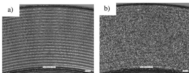
Fig. 10. Macrostructure of the cast iron ring insert: before shot blasting with visible traces of machining a); after shot blasting b)
