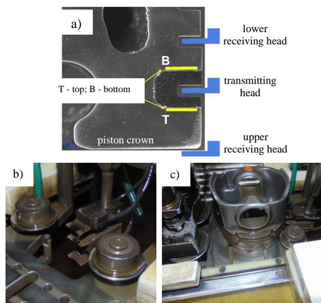
Fig. 4. Method of measuring connections between the insert and the piston: arrangement of measuring heads a); measuring stations b, c)
