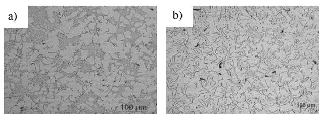
Fig. 9. Microstructure of EN-GJLA-XNiCuCr15-6-2 cast iron: not consistent with the standard a); consistent with ISO 945-1:2008 b)
