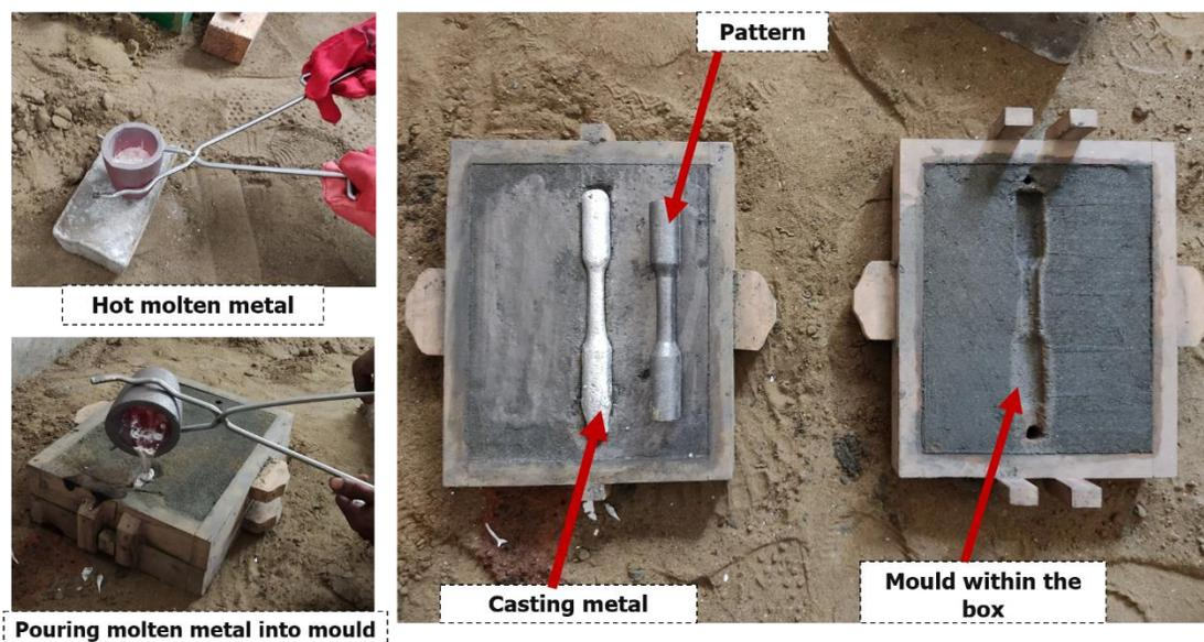
Fig. 6. Processes of casting using river sand as a mould material
