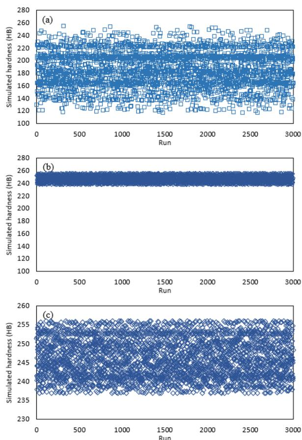
Fig. 4. Variations of simulated hardness values after performing MCS on different proportions of components for (a) previous constraints (b) and (c) for appropriate proportion of the four components
