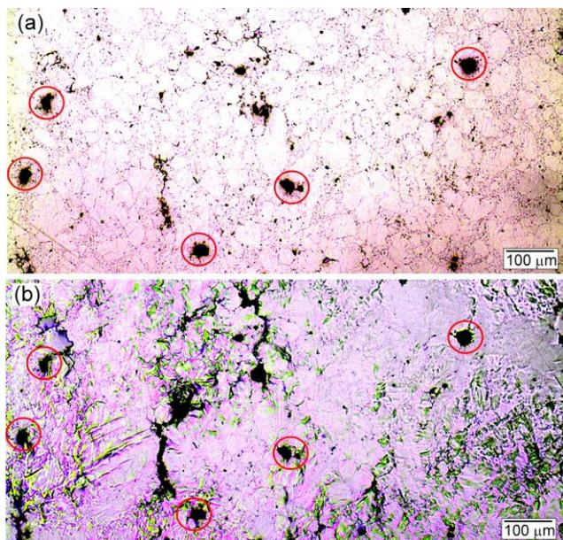
Fig. 4. Same hpdc AME501 alloy sample surface before (a) and after 8% deformation (b); light microscopy
