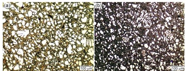
Fig. 2. Microstructure of cold-chamber die-cast AME501 (a) and AME505 (b) magnesium alloys; light microscopy
