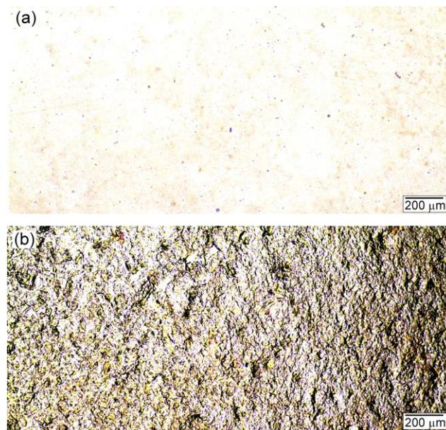
Fig. 5. Same hpdc AME505 alloy sample surface before (a) and after 8% deformation (b); light microscopy
