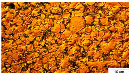
Fig. 8. Microstructure of hpdc AME505 alloys sample after 8% deformation; light microscopy with differential interference contrast
