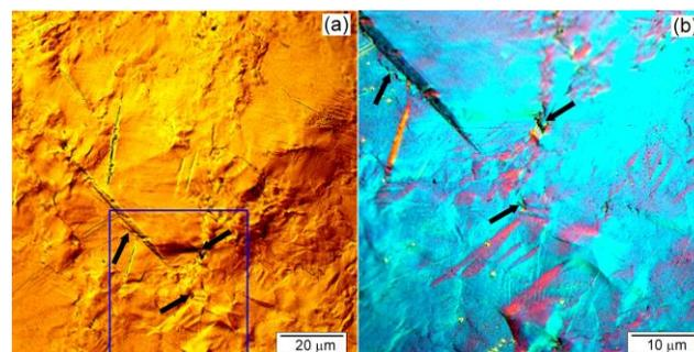
Fig. 6. Hpdc AME501 alloys sample surface after 8% deformation (a) and higher magnification of area marked by navy blue square (b); light microscopy with differential interference contrast
