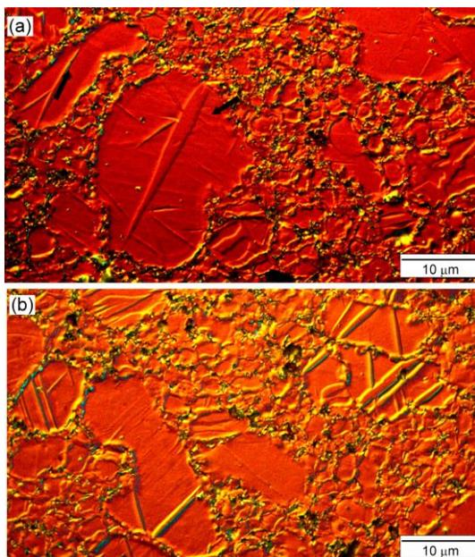
Fig. 7. Microstructure of hpdc AME503 alloys sample after 8% deformation; light microscopy with differential interference contrast
