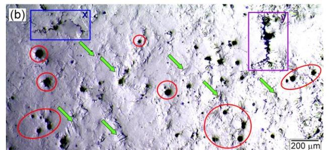
Fig. 3. Same hpdc AME501 alloy sample surface before (a) and after 6% deformation (b); light microscopy
