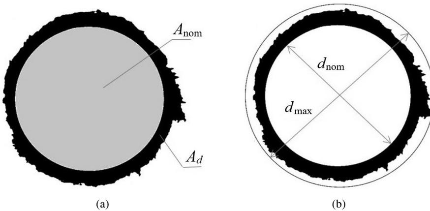
Fig. 6. Definition of delamination factors (a)  $F_a$  and (b)  $F_d$
