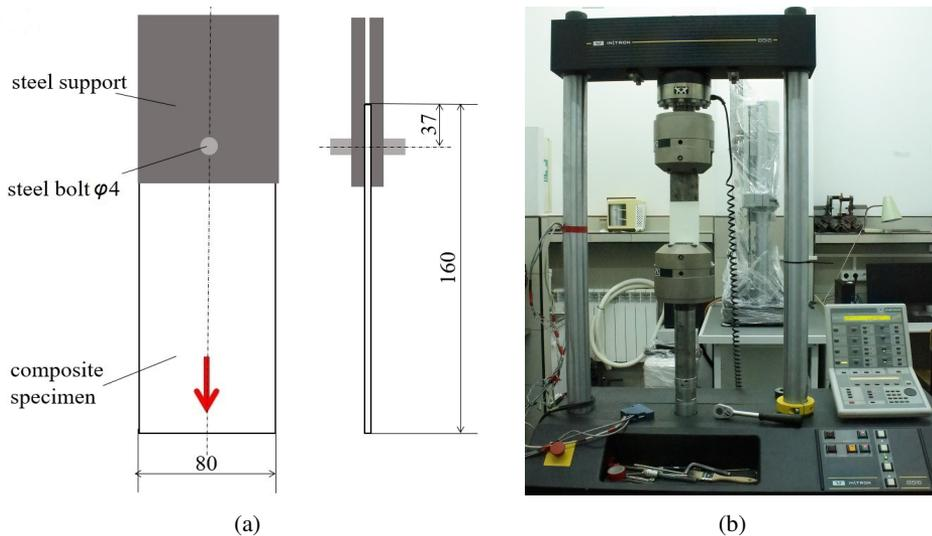
Fig. 9. SLS specimen scheme (a) and experimental set-up (b)
