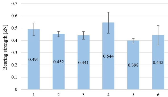
Fig. 10. Bearing strength results for holes made by different drills: plain HSS (drill 1), HSS with 5% addition of cobalt, (drill 2), HSS with 5% addition of cobalt with titanium coating (drill 3), HSS with titanium coating (drill 4), cemented carbide (drill 5) and HSS tipped with tungsten carbide (drill 6)
