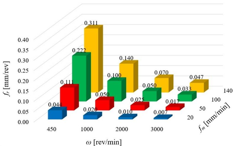
Fig. 2. Graph of  $f_r$  feed for all sets of drilling parameters
