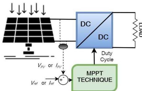
Fig. 7. Voltage/current feedback method
