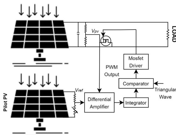
Fig. 4. PV pilot concept
