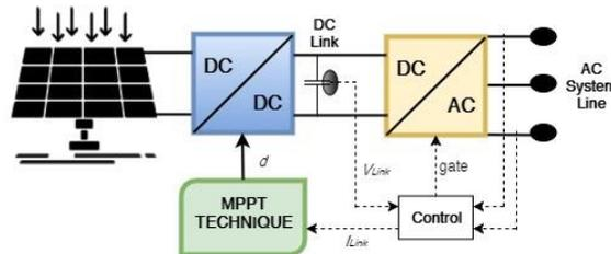
Fig. 13. DC-link capacitor drops control method diagram
