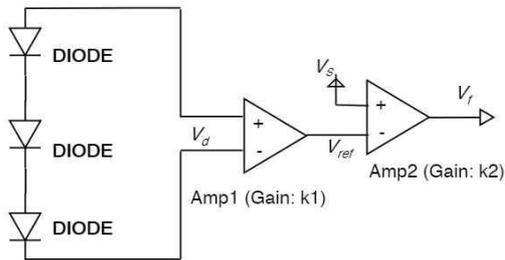
Fig. 9. Control circuit configuration based on constant voltage
