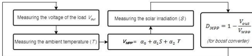
Fig. 6. Improved temperature parametric algorithm
