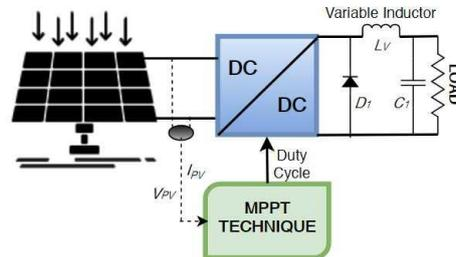
Fig. 14. Variable inductance method diagram
