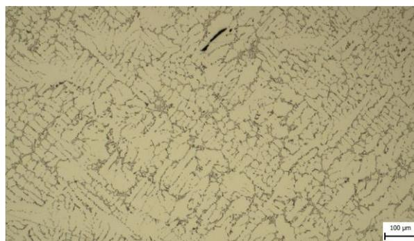
Fig. 3 Microstructure AlSi7Mg0.3 in cast state – 300
