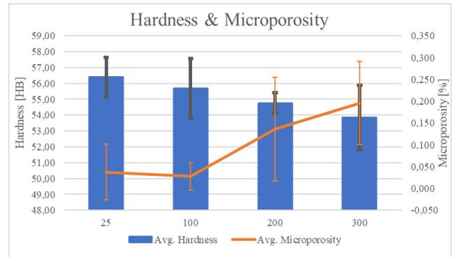
Fig. 4 Comparison of hardness and microporosity values
