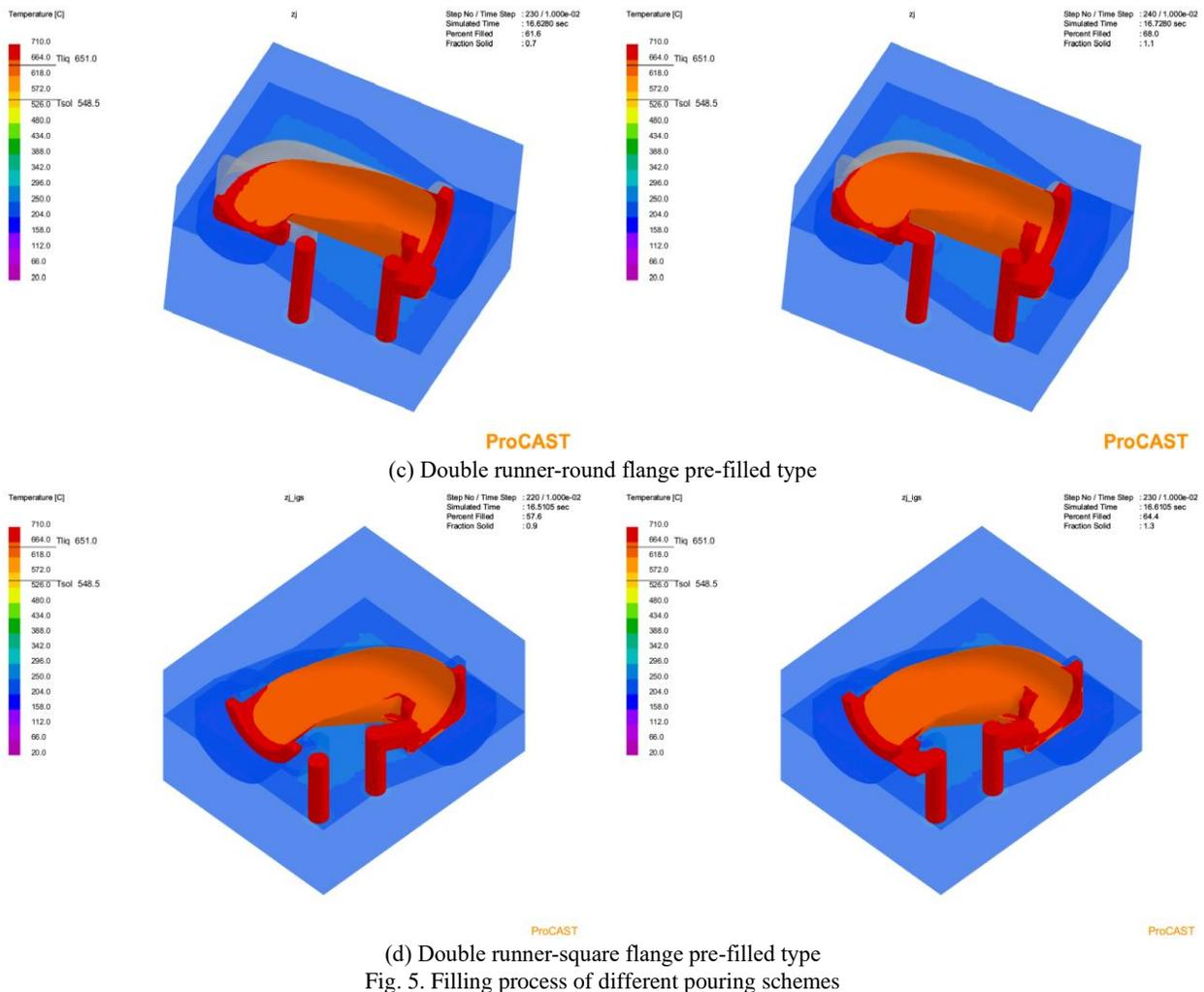
Fig. 5. Filling process of different pouring schemes
