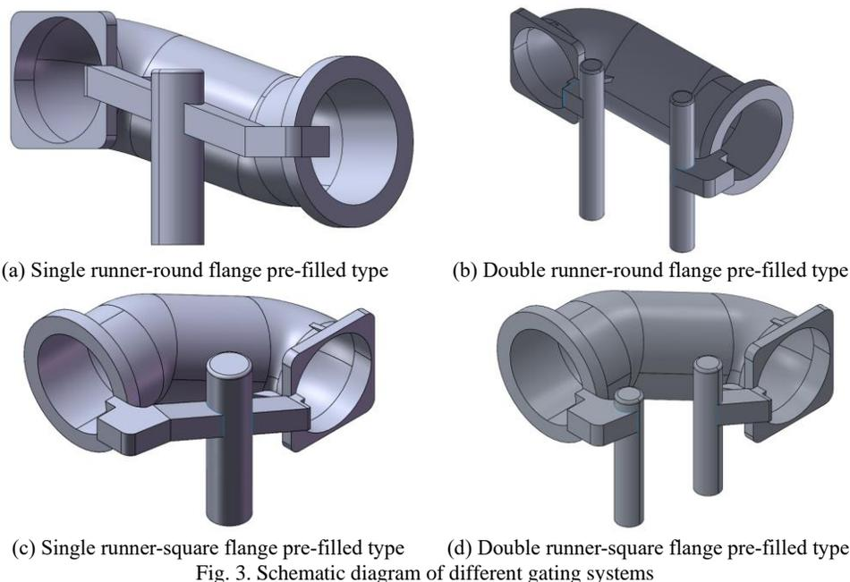
Fig. 3. Schematic diagram of different gating systems
