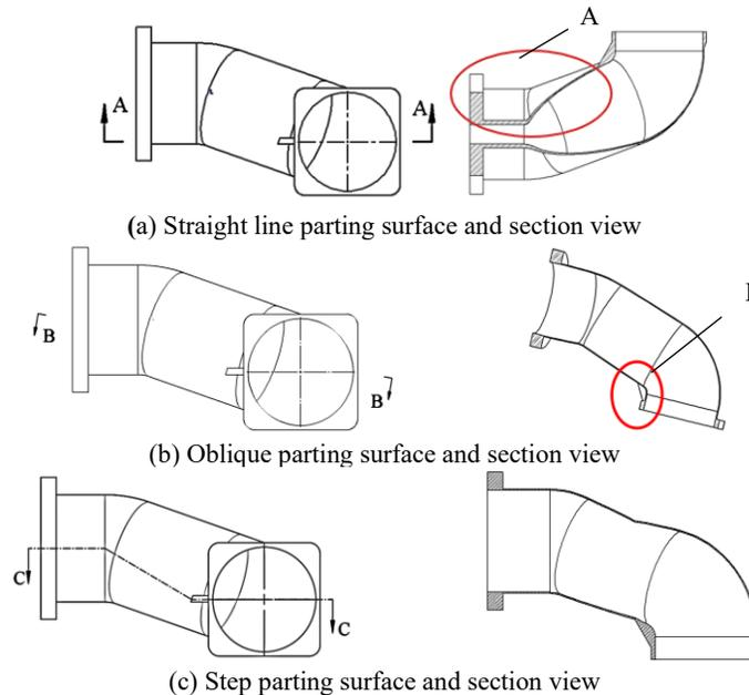
Fig. 2. Parts parting surface selection
