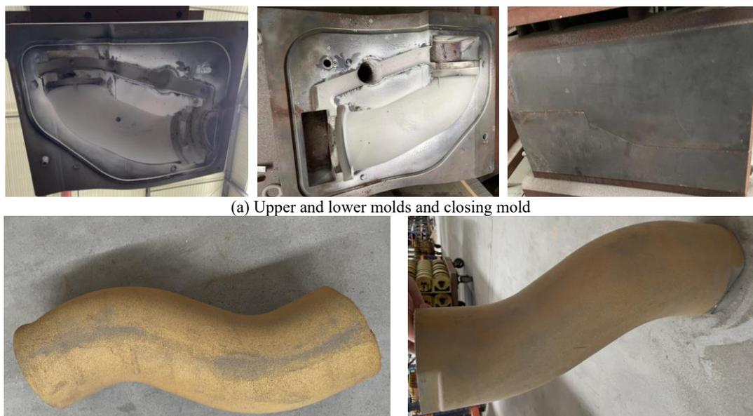
(a) Upper and lower molds and closing mold
