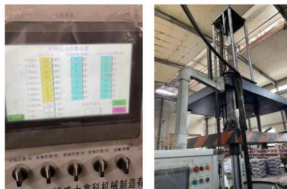
Fig. 13. Low-pressure casting equipment and actual parameter settings
