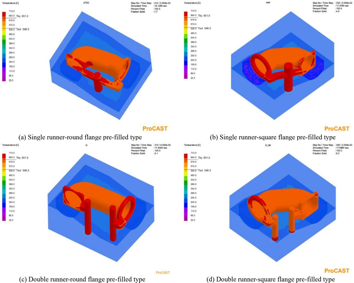
Fig. 6. Temperature distribution of different pouring schemes
