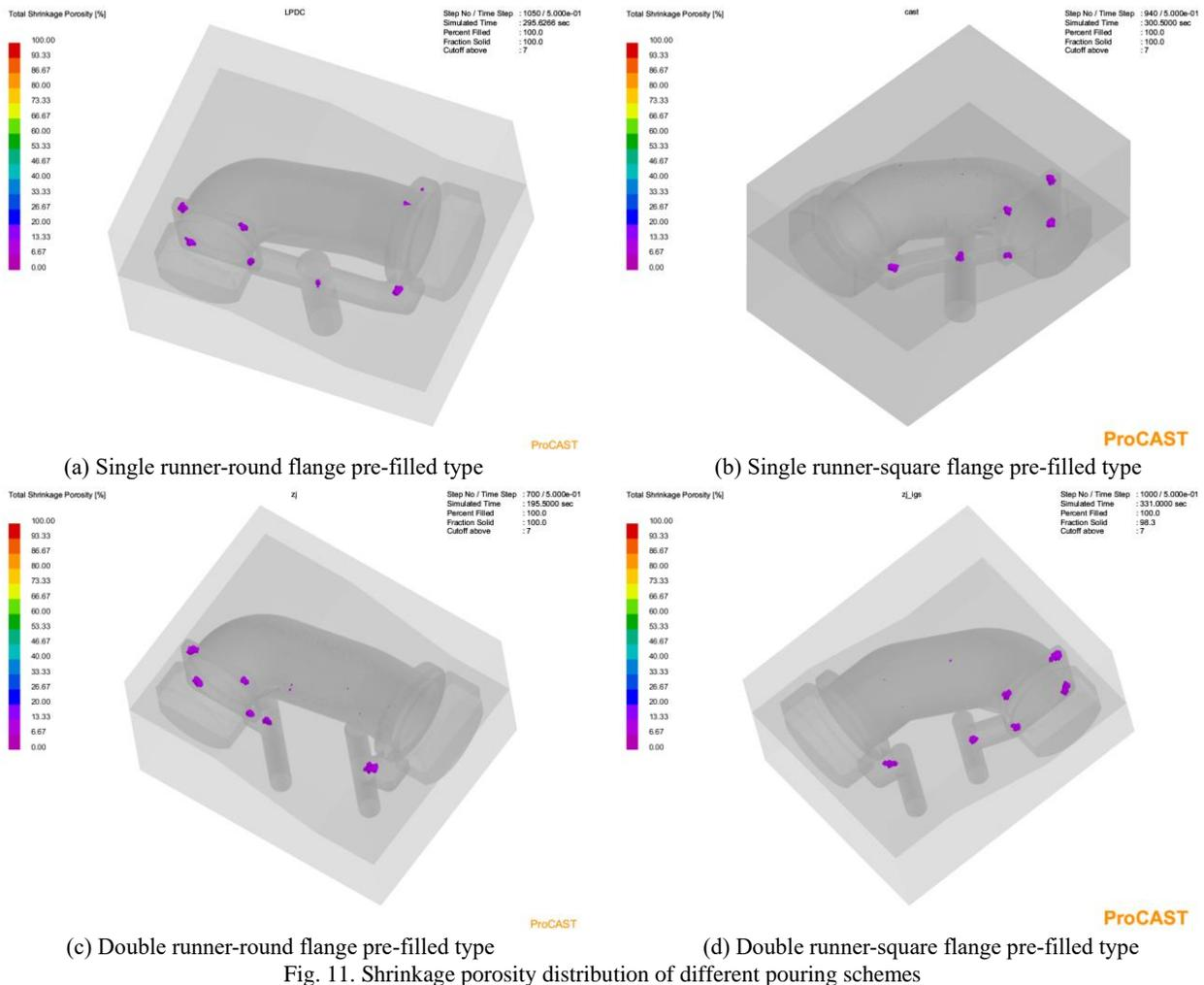
Fig. 11. Shrinkage porosity distribution of different pouring schemes
