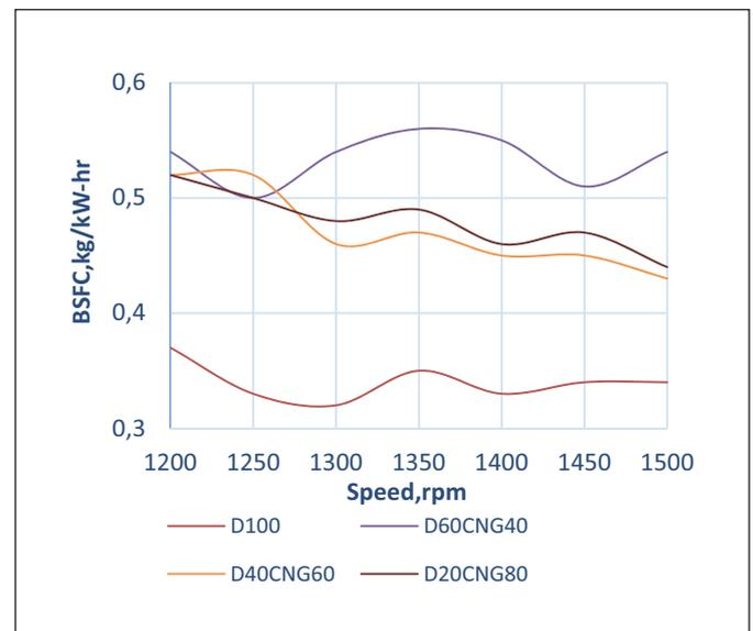
Fig. 3. Variation of brake specific fuel consumption versus engine speed
