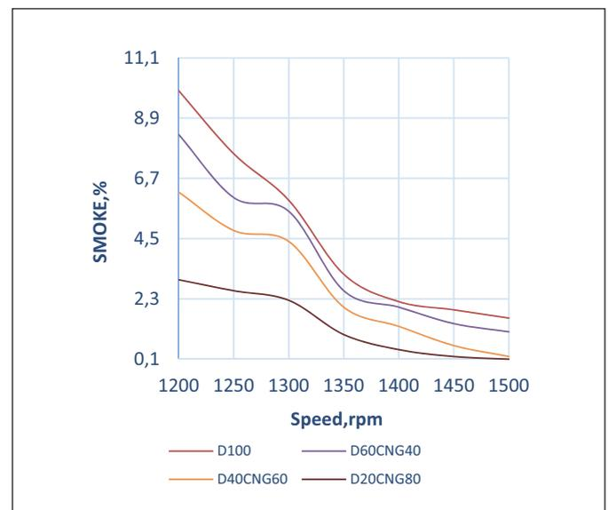
Fig. 7. Variation of Smoke opacity versus engine speed
