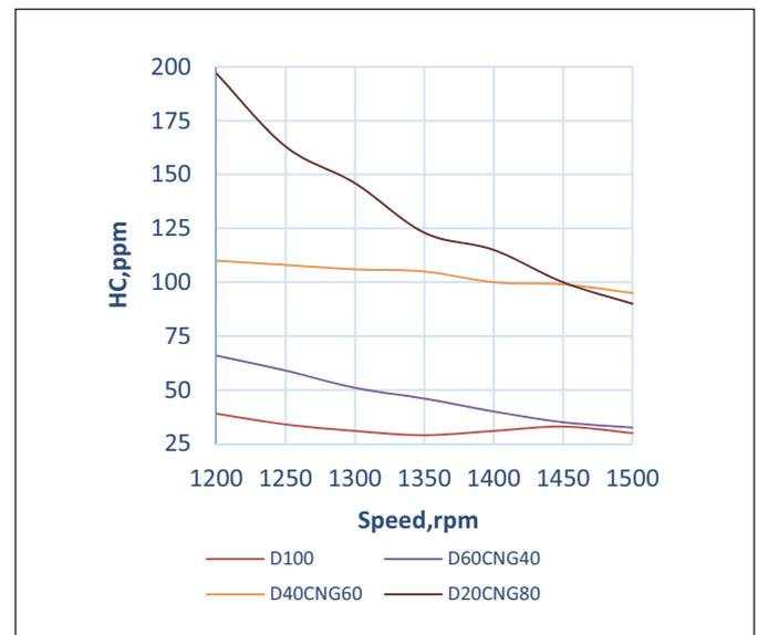
Fig. 5. Variation of HC emission versus engine speed
