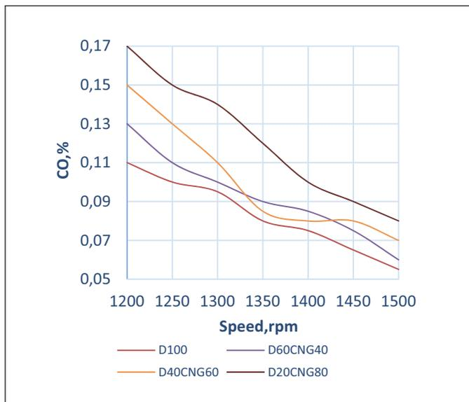
Fig. 4. Variation of CO emission versus engine speed
