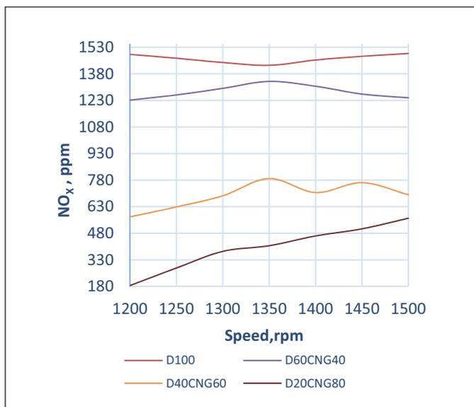
Fig. 6. Variation of  $\text{NO}_x$  emission versus engine speed
