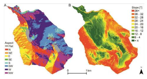
Fig. 6. Aspect (A) and slope (B) in the Bratteggelva catchment, based on digital elevation model.
