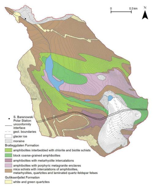
Fig. 2. Geological map of the study area modified from Czerny *et al.* (1993). Note different extent of the glacier and lakes as compared to Fig. 1, which is due to considerably earlier time of mapping.
