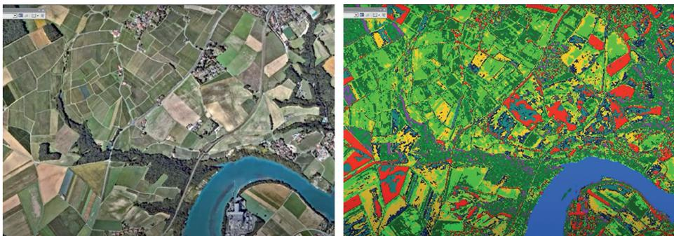
Fig. 12. Classification for impervious surfaces with machine learning SVM method
