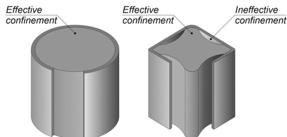
Fig. 1. Confinement effect in aluminium-concrete columns [38]
