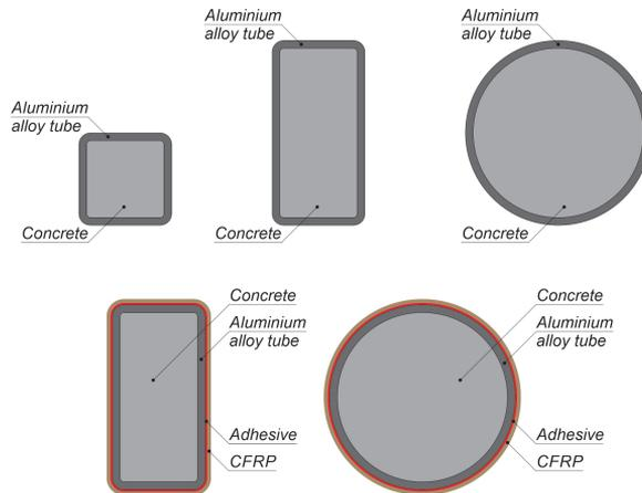
Fig. 2. Aluminium-concrete columns [37, 38, 41, 42, 46]
