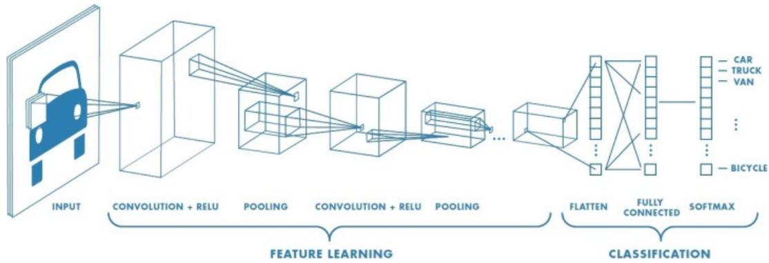
Fig. 3. CNN Architecture
