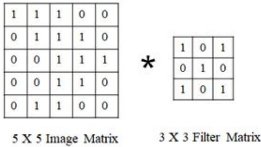
Fig. 4. Multiplication of Image matrix and Filter matrix
