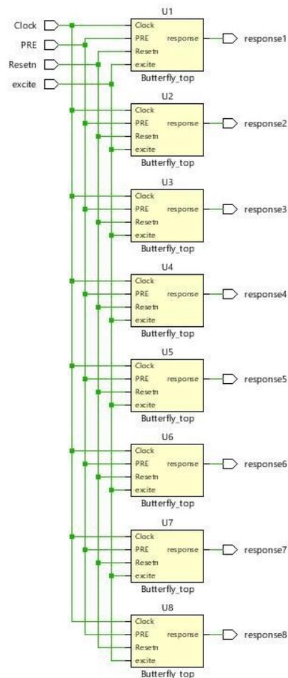
Fig. 3. RTL of the proposed modified butterfly PUF
