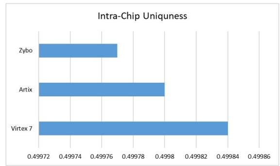
Fig. 6a. Intra chip uniqueness in different FPGAs
