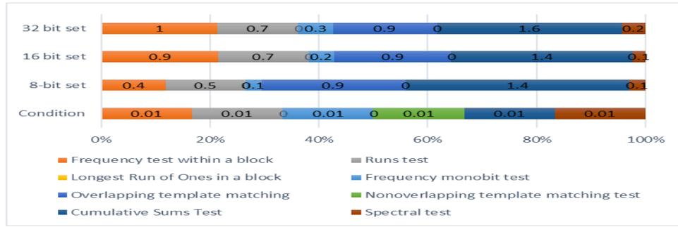
Fig. 4. NIST Test Results of PUF based TRNG
