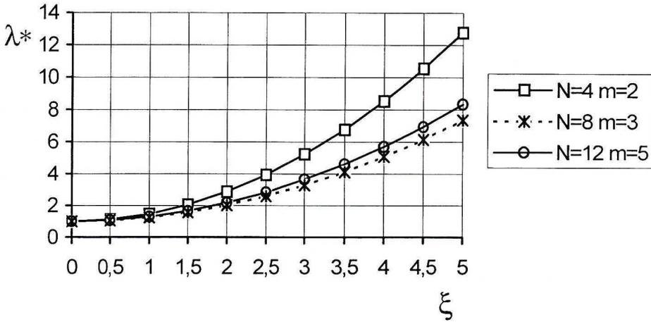
Fig. 9. Postbuckling equilibrium paths for columns with non-stiffened walls (uncoupled stability)
