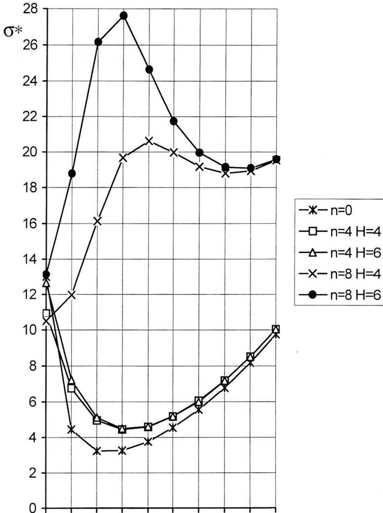
Fig. 8. The influence of intermediate stiffeners on critical stress values for columns with octagonal cross-section (for three values of orthotropy factor  $\eta$ )
