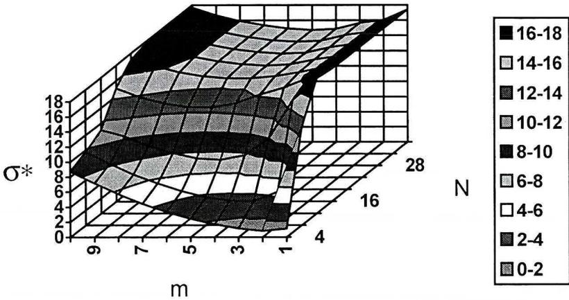
Fig. 3. Dimensionless critical stress for non-stiffened tubular columns
