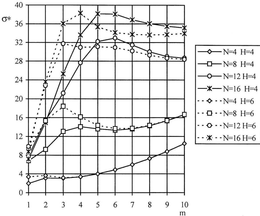
Fig. 6. Dimensionless critical stress versus number of half-waves for isotropic tubular poles of walls number  $N$  with one central stiffener placed on each wall ( $N=n$ )
