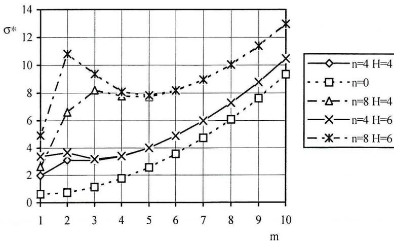
Fig. 5. The influence of intermediate stiffeners on values of critical stress for isotropic column of a square cross-section
