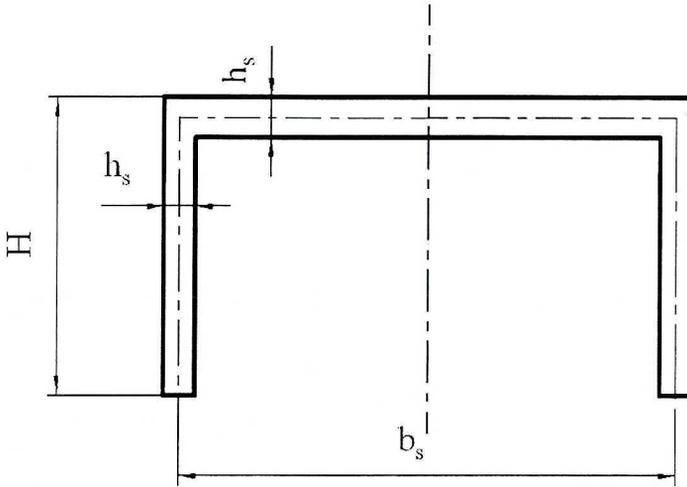
Fig. 4. Shape of stiffener cross-section -  $h_s=1$  mm,  $b_s=4$  mm,  $H=4$  or  $6$  mm
