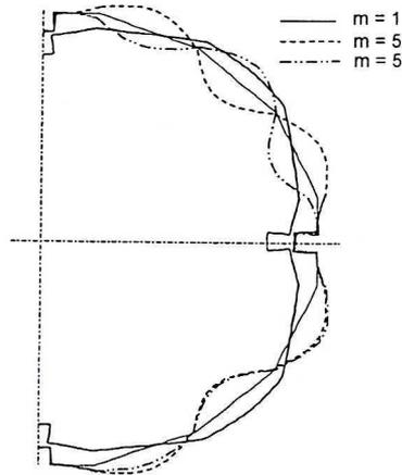
Fig. 7a. Shapes of buckling modes for isotropic column with four intermediate stiffeners (number of walls  $N=16$ )
