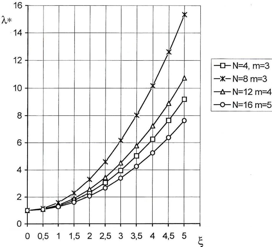
Fig. 10. Postbuckling equilibrium paths for stiffened (4 intermediate stiffeners) columns (uncoupled stability)
