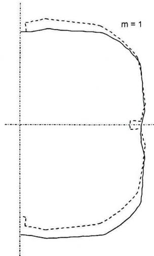
Fig. 7b. Comparison of buckling mode shapes ( $m=1$ ) for isotropic column with four intermediate stiffeners (dotted line) and without stiffeners (full line) - number of walls  $N=16$
