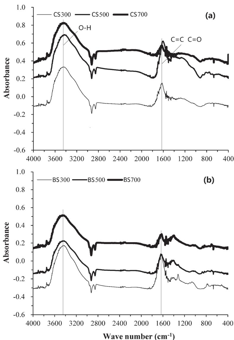
**Fig. 1.** The infrared spectra of biochar at different pyrolysis temperatures. CS300, CS500 and CS700 denote coconut shell biochar derived at 300, 500 and 700°C, respectively; BS300, BS500 and BS700 denote banana stem biochar derived at 300, 500, and 700°C, respectively
