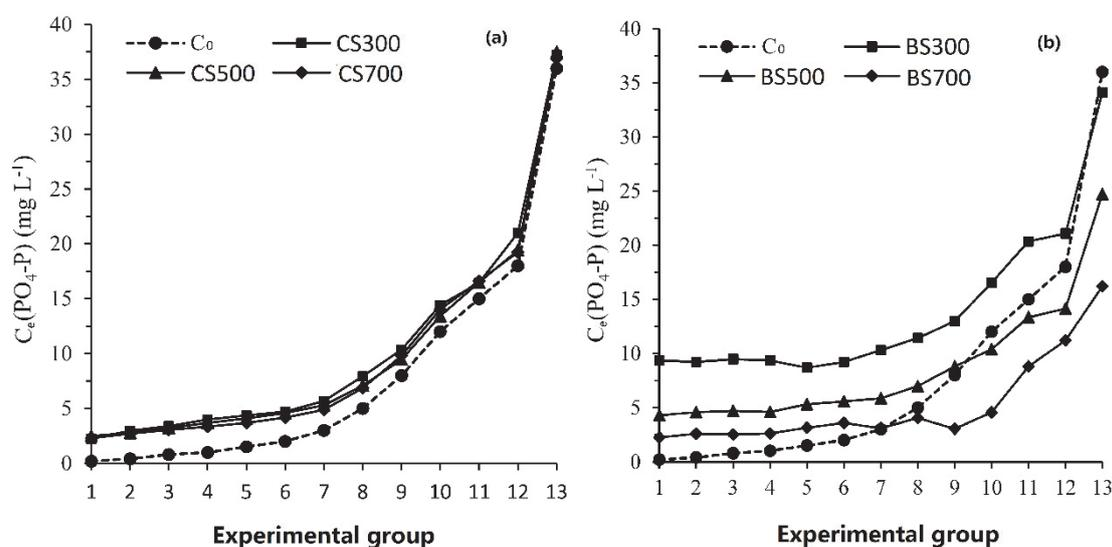
**Fig. 4.** The comparison of phosphate concentration in water between equilibrium state and initial state with different biochars. CS300, CS500, and CS700 denote coconut shell biochar derived at 300, 500, and  $700^\circ\text{C}$ , respectively; BS300, BS500, and BS700 denote banana stem biochar derived at 300, 500, and  $700^\circ\text{C}$ , respectively. The  $C_e$  and  $C_0$  refers to the equilibrium and initial phosphate concentration of aqueous solution, respectively.
