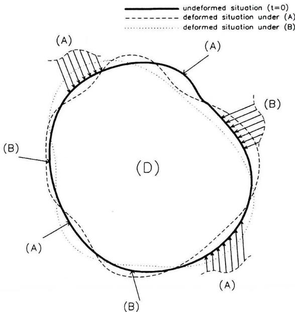
Fig. 2. Elastic body (D) subjected to the systems of external actions (A) or (B)
