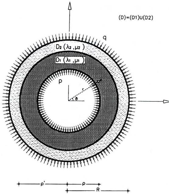
Fig. 4. A two material cylindrical pipe under uniform internal and external pressure
