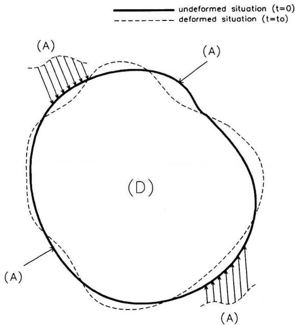
Fig. 1. Elastic body (D) subjected to the system of external actions (A)
