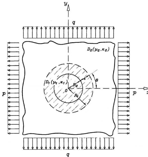
Fig. 5. Stretching of an infinite plate with an inserted elastic disc
