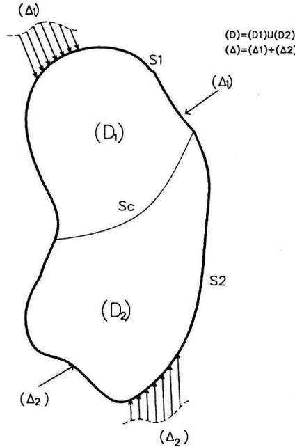
Fig. 3. A system (D) of two elastic bodies subjected to the external actions  $(\Delta)$
