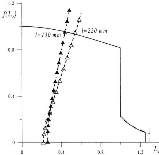
Fig. 2.5. FAD's for the straight segment with a through-the-thickness crack for virgin material ( $\Delta$ ) and after 156000 hours of service ( $\blacktriangle$ )
