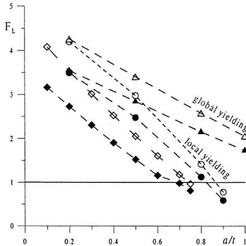
Fig. 2.3. Reduction of the sensitivity coefficient  $F_L$  for various crack shapes (semi-elliptical surface crack: virgin material –  $\circ$ ,  $\Delta$  and material after 156000 hours operation –  $\bullet$ ,  $\blacktriangle$ ; infinite surface crack: virgin material –  $\diamond$  and material after 156000 hours operation –  $\blacklozenge$ )
