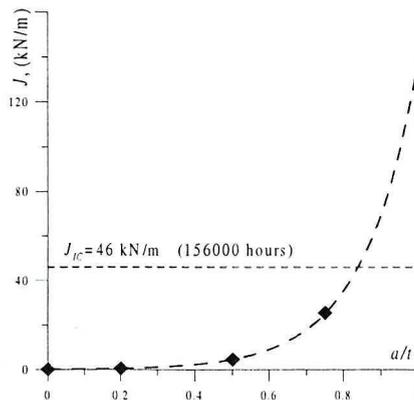
Fig. 4.1. Estimation of safety of the straight pipeline element with inner-axial-infinite crack according to procedure in [14]
