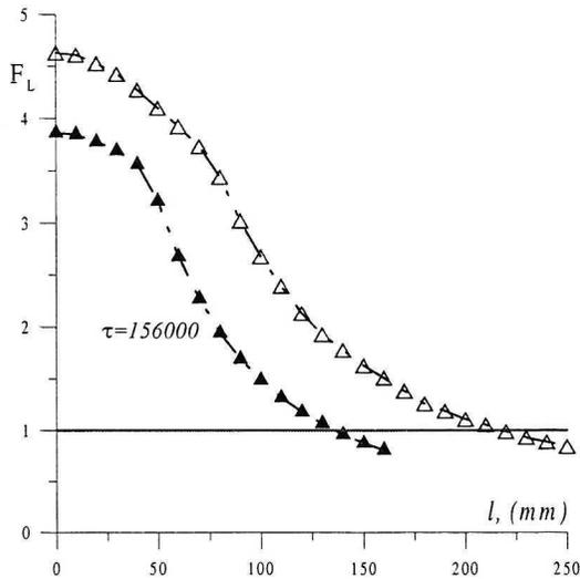
Fig. 2.6. The plot of the sensitivity coefficient  $F_L$  v.s. crack length  $l$ . ( $\Delta$  - virgin material,  $\blacktriangle$  - after 156000 hours of service)
