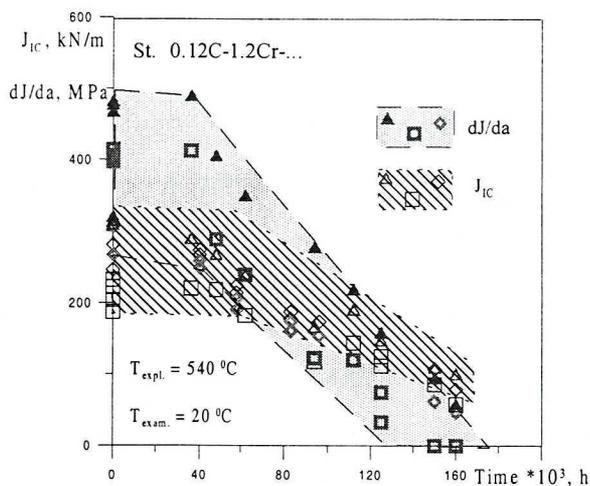
Fig. 1.2. The change of the fracture toughness parameters  $J_{IC}$  and  $dJ/da$  during operation time
