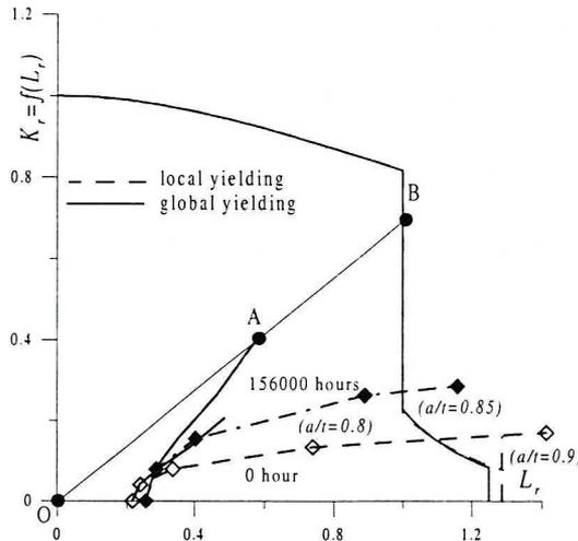
Fig. 2.1. FAD's for finite-axial-internal surface, semi-elliptic crack
