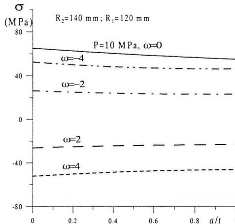
Fig. 3.1. The hoop stress distribution in the wall of pipeline due to the temperature gradients for various rates  $\omega$  of cooling or heating (dashed lines) and stationary regime  $\omega = 0$  (solid line)
