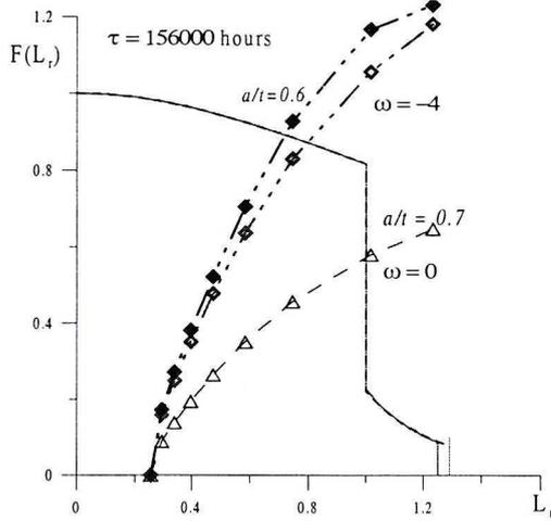
Fig. 3.2. The FAD's for straight pipeline element with axial inner infinite crack for cooling process ( $\omega = -4$ ,  $\blacklozenge, \hat{\lozenge}$ ) and stationary regime ( $\triangle, \hat{\triangle}$ ) ( $\blacklozenge, \hat{\lozenge}$  – with correction function  $\rho(a)$ ,  $\hat{\lozenge}, \hat{\triangle}$  – without correction function  $\rho(a)$ )
