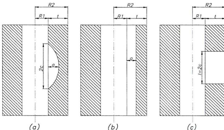
Fig. 1.4. Cracks analysed in the paper: (a) – finite-axial-internal surface semi-elliptic crack; (b) – infinite-axial-internal surface crack; (c) – axial-through-thickness crack
