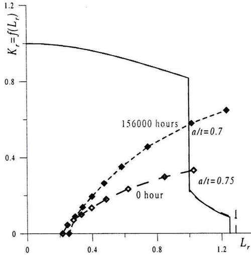
Fig. 2.2. FAD's for infinite-axial-internal surface crack
