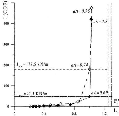
Fig. 2.4. CDF diagrams for axial-inner surface crack of infinite length
