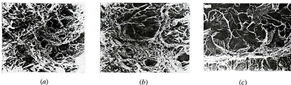
Fig. 1.3. Fracture mechanisms at the initial stage of crack propagation for 12Kh1MF steel at various period of service: (a) ductile – before service; (b) mixed, the regions of ductile fracture are followed by the regions of cleavage fracture – after 125000 hours of operation; (c) cleavage – after 156000 hours of operation. The arrows indicate direction of the crack propagation
