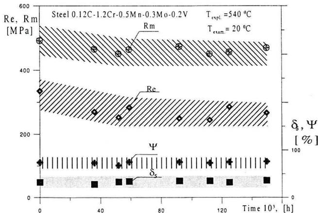
Fig. 1.1. The range of the mechanical properties of the 12Kh1MF steel during operation time
