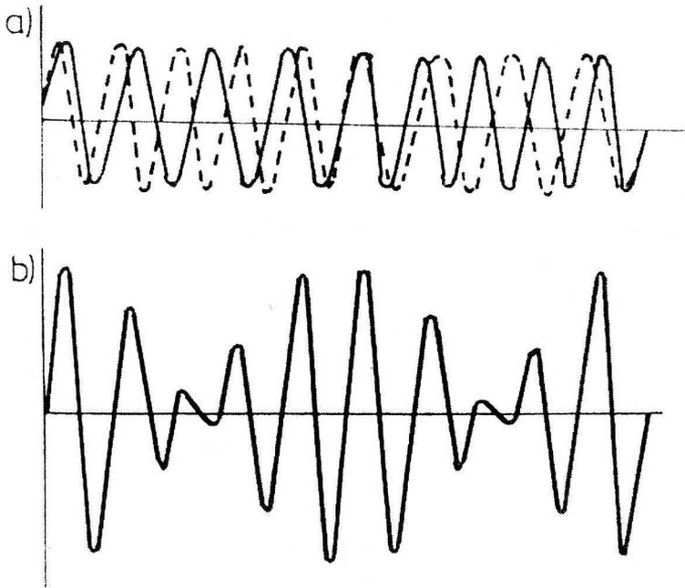
Fig. 2. a) Two pulsation waves of the same amplitude, b) Resultant pressure wave
