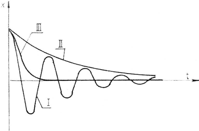
Fig. 5. Damped vibration I – damped vibration ( $\omega_0^2 - \beta^2 > 0$ ), II – aperiodic vibrations ( $\omega_0^2 - \beta^2 < 0$ ), III – damped, critical vibrations ( $\omega_0^2 - \beta^2 = 0$ )
