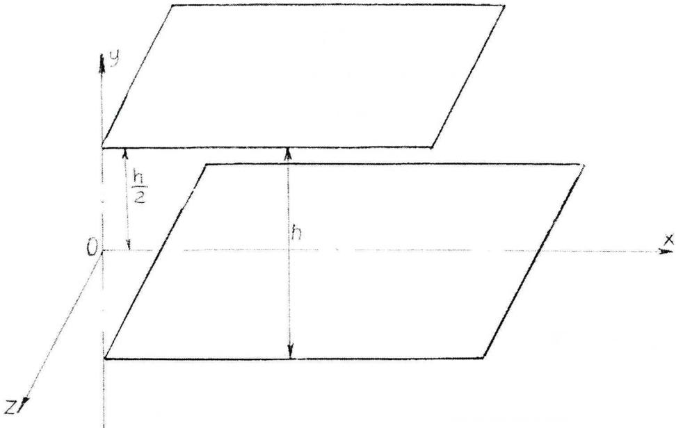
Fig. 8. Diagram of flow between two parallel, stationary planes
