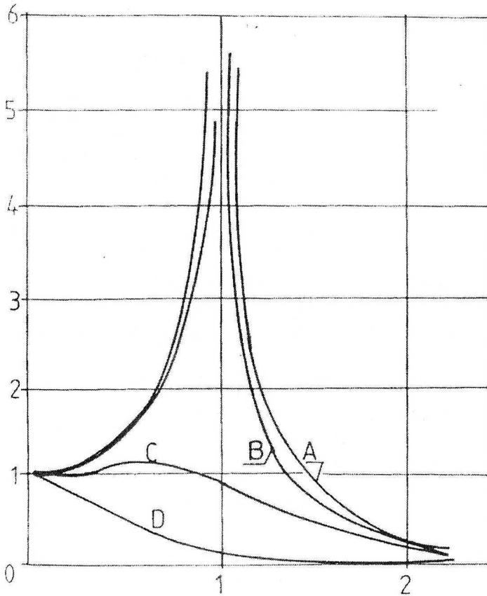
Fig. 6. Dependence of the vibration amplitude on the frequency of vibrations forced for the various values the decay constant ( $A < B < C < D$ )
