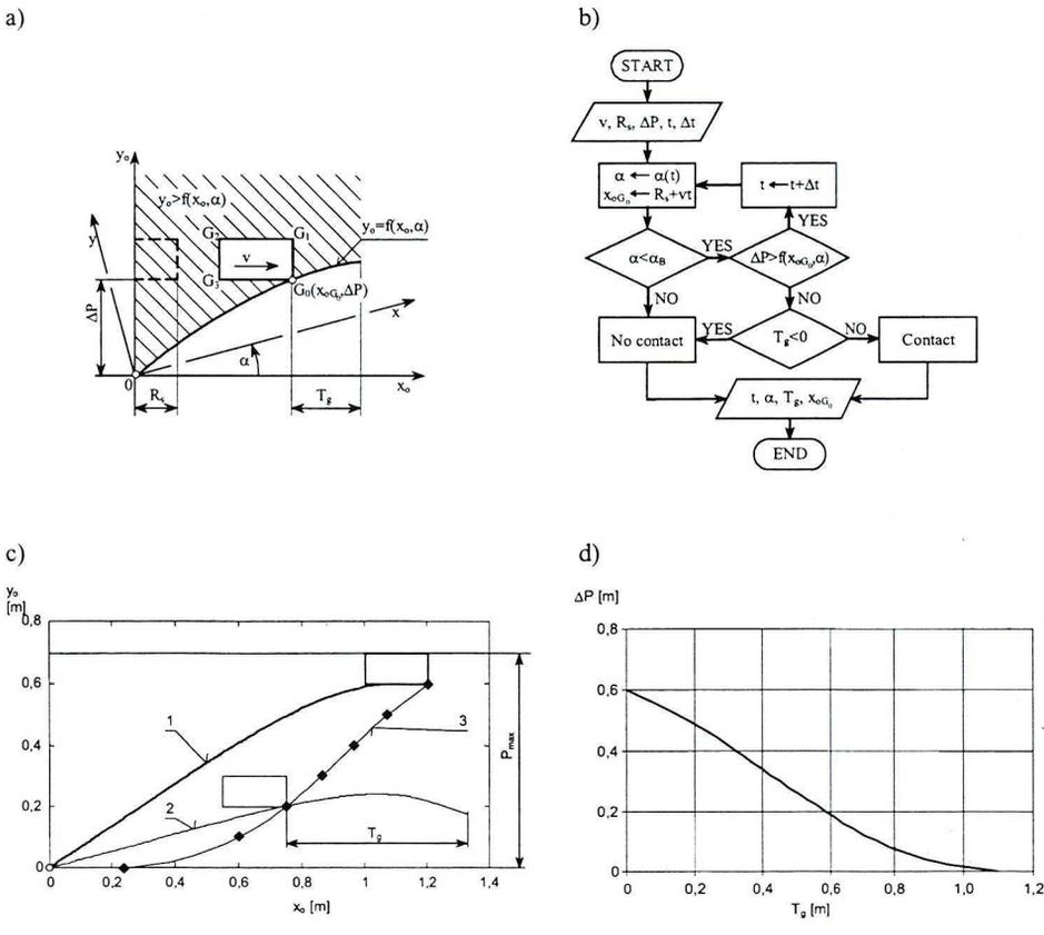
Fig. 9. Conditions for the occurrence of contact between the load and the scraper: a) graphical interpretation, b) numerical algorithm, c) the scraper arm and the load position at the moment of contact (1 – for  $\Delta P = 0,6$  m, 2 – for  $\Delta P = 0,2$  m, 3 – curve determining contact points between the load and scraper,  $T_g$  – distance between the load point contact with the scraper and the end of the scraper arm), d) chart  $\Delta P$  in function  $T_g$
