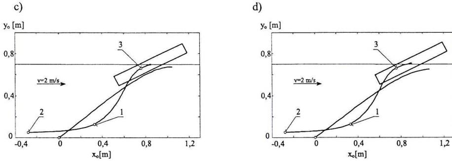
Fig. 11. Path of the load centre of gravity: a), b), c), d) – load and scraper arm positions determined for time range  $\Delta t = 0.03$  s; 1, 2, 3 – load characteristic motion stages
