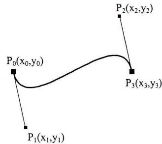
Fig. 2. Bézier's curve,  $n=3$ : a) three dimensional system, b) two dimensional system
