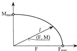
Fig. 6. Limit surface of the friction
