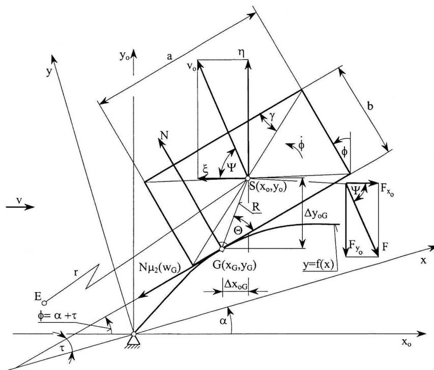
Fig. 8. Scheme of the load motion along the rotating scraper arm
