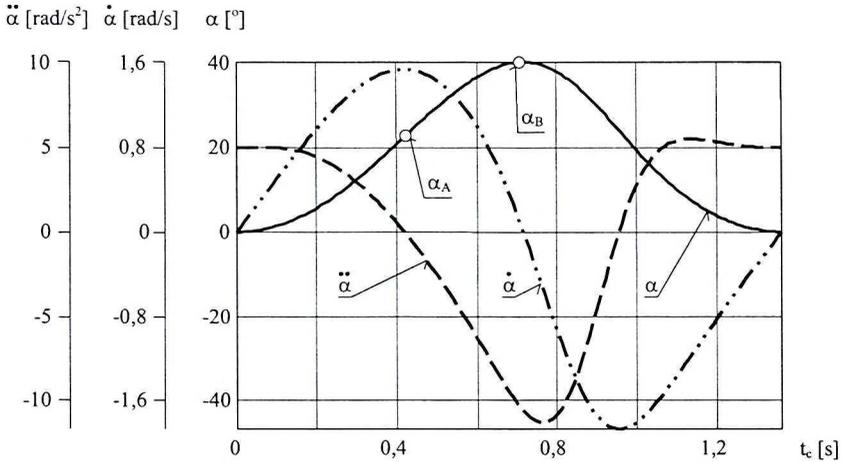
Fig. 4. Characteristic of kinematical motion of scraper arm
