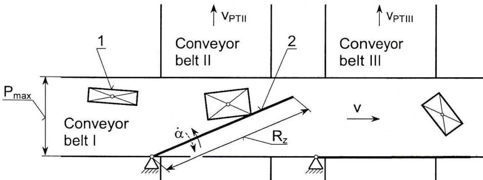
Fig. 1. Divider with the deflection scraper arm: 1 – unit load, 2 – scraper arm,  $P_{max}$  – conveyor width,  $R_z$  – arm length,  $v$ ,  $v_{PTII}$ ,  $v_{PTIII}$  – conveyor linear velocity
