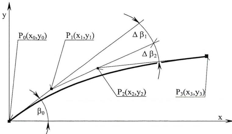
Fig. 5. Requirements concerning scraper arm geometry (polygon determined through the control and extreme points)
