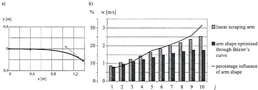
Fig. 10. Research results: a) proposed scraper arm shape, b) chart of relative velocities in normal impact direction  $w_j$  according to ten test points
