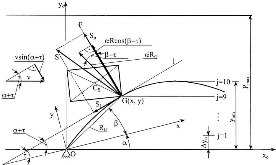
Fig. 3. Oblique impact between the unit load and the curvilinear scraper arm
