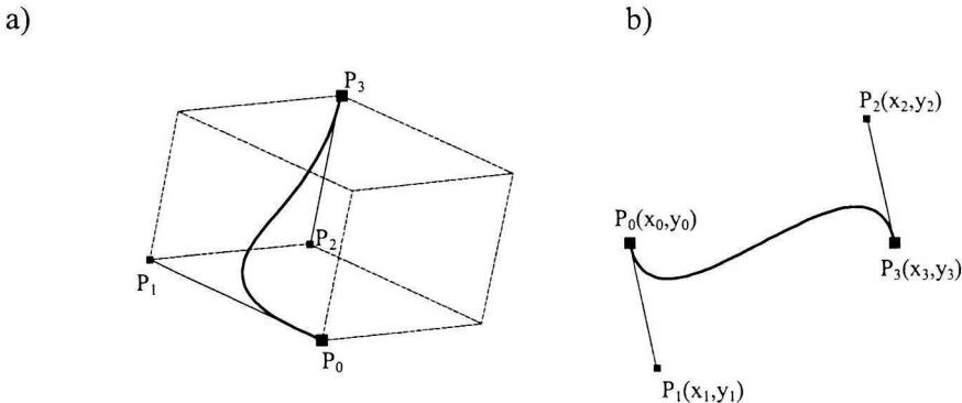
Fig. 2. Bézier's curve,  $n=3$ : a) three dimensional system, b) two dimensional system
