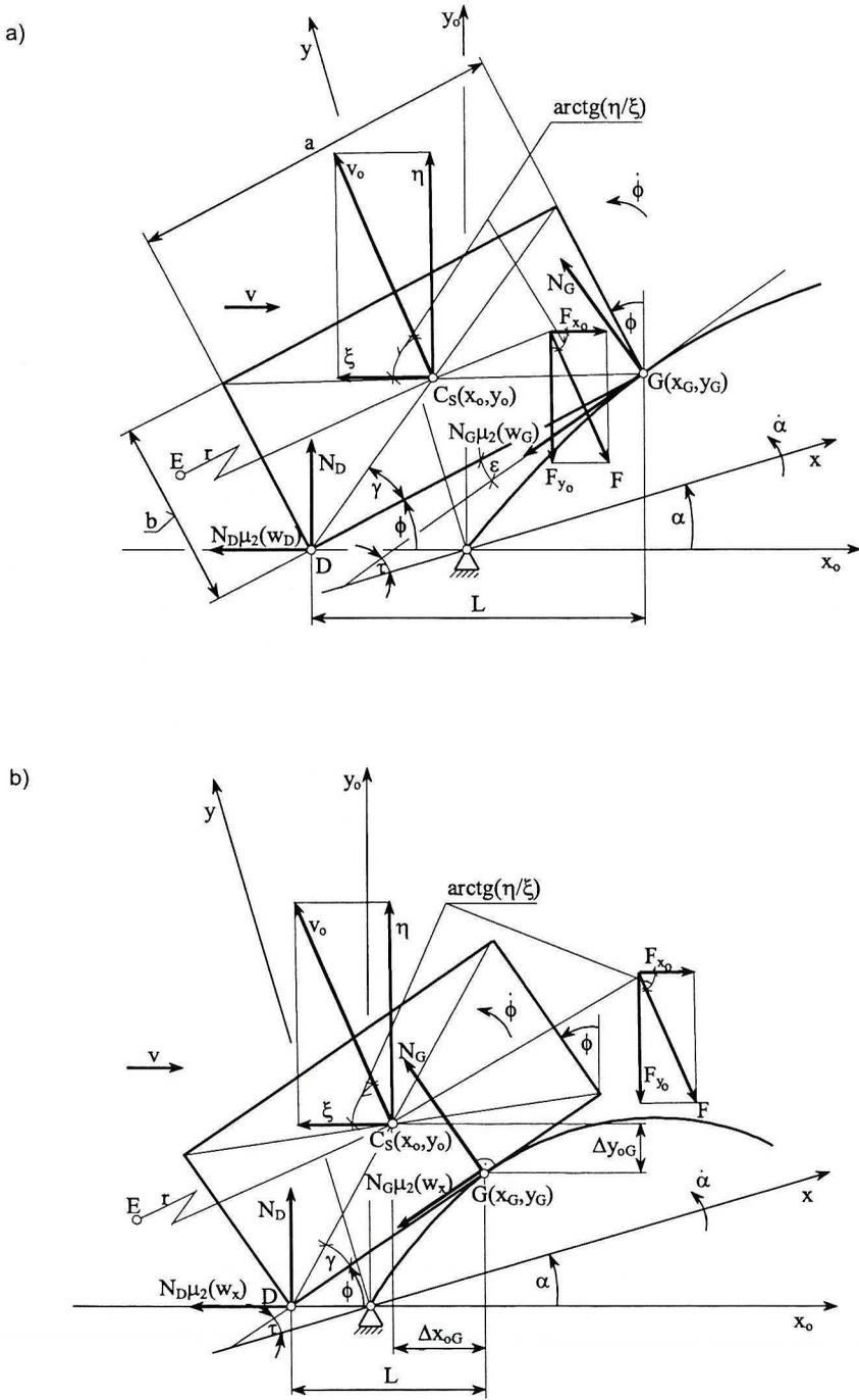
Fig. 7. Scheme of the load motion placed at the conveyor belt edge sliding against the conveyor side and the scraper arm: a) with the load corner, b) with the load side
