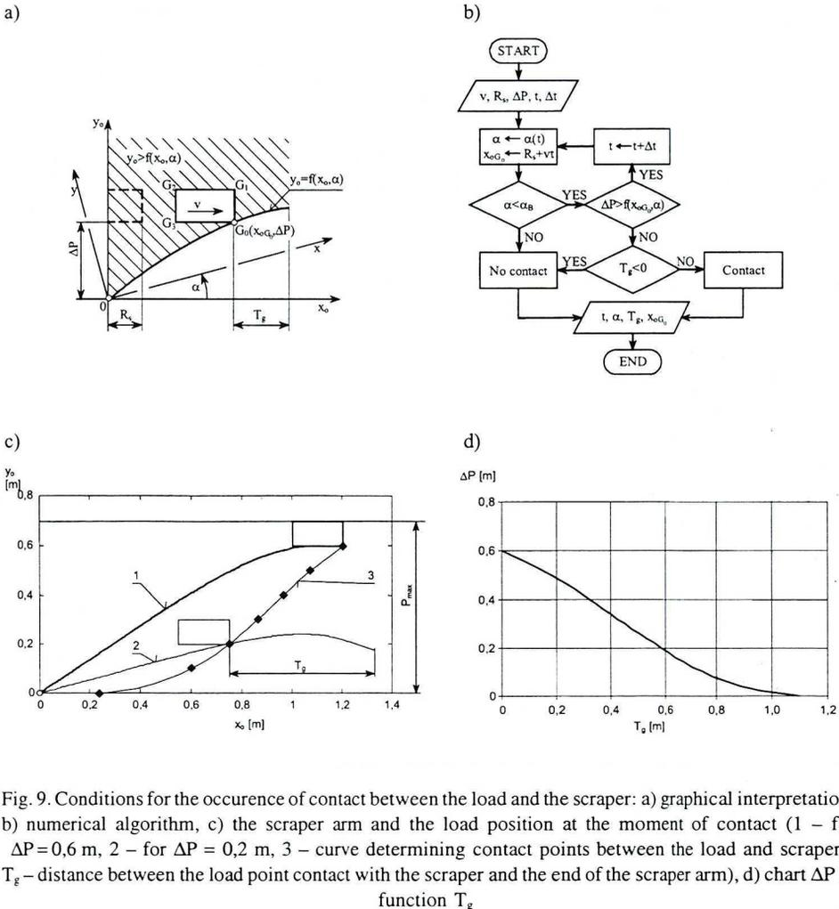
Fig. 9. Conditions for the occurrence of contact between the load and the scraper: a) graphical interpretation, b) numerical algorithm, c) the scraper arm and the load position at the moment of contact (1 – for  $\Delta P = 0,6$  m, 2 – for  $\Delta P = 0,2$  m, 3 – curve determining contact points between the load and scraper,  $T_g$  – distance between the load point contact with the scraper and the end of the scraper arm), d) chart  $\Delta P$  in function  $T_g$
