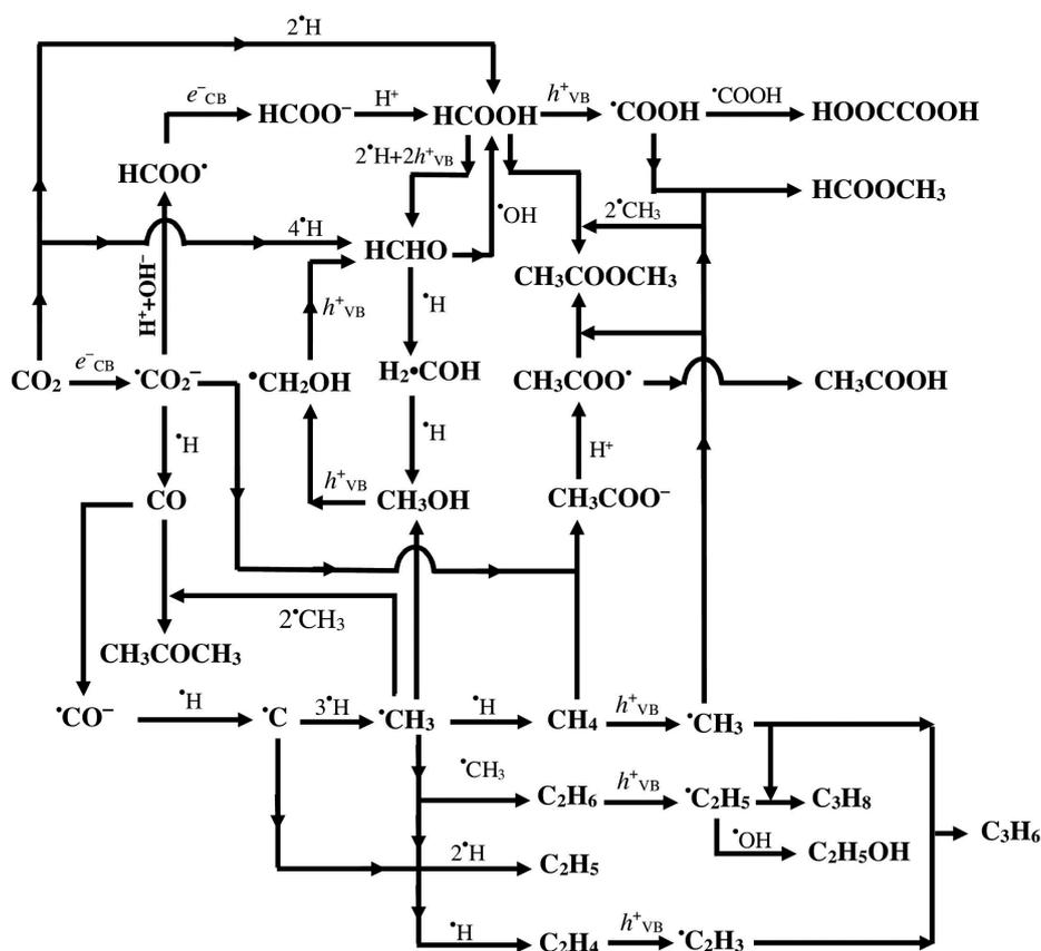
Fig. 3. Representation of mechanisms for reducing CO<sub>2</sub> with the use of different catalysts, with a couple of possible pathways. Reprinted from (Karamian and Sharifnia, 2016) with permission of Elsevier Ltd.
