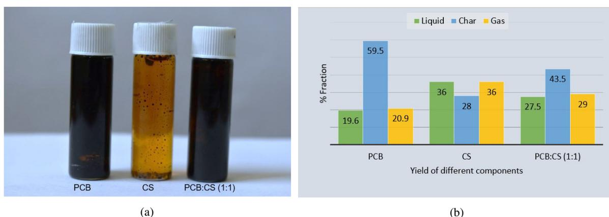
Fig. 2. (a) Appearance of generated oil with different feedstock; (b) different feedstock with generated amount of liquid oil, solid char and gas in percentage
