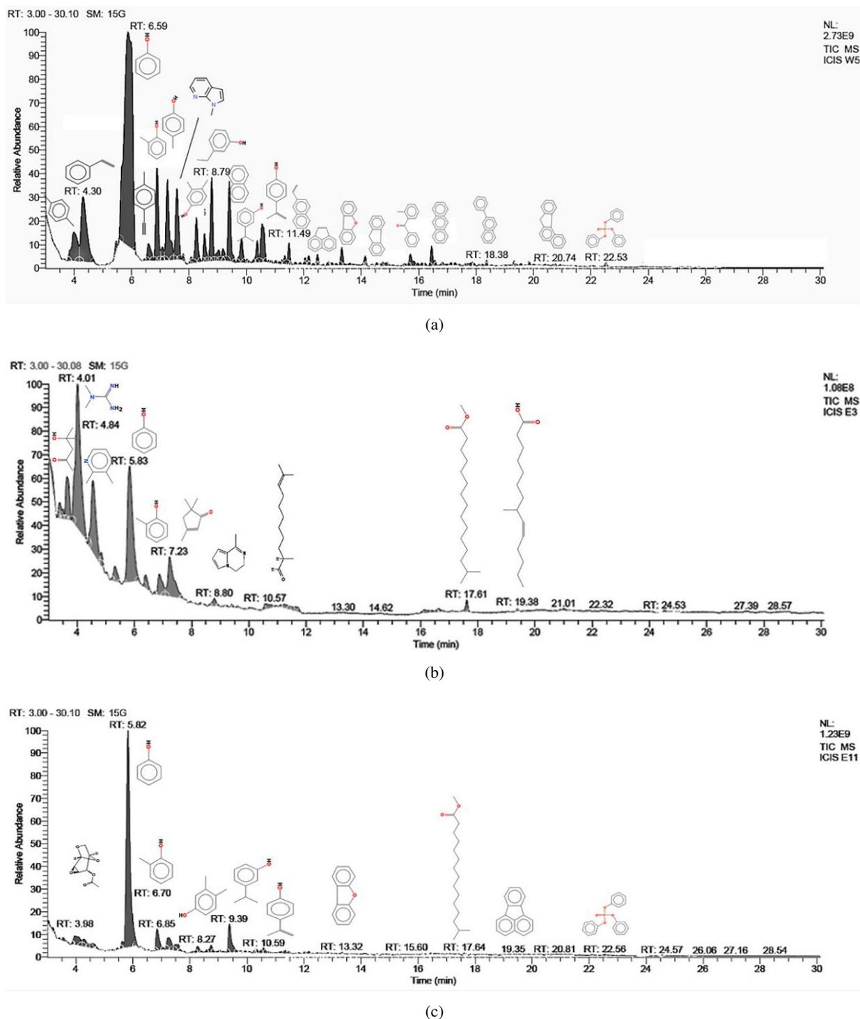
Fig. 4. GC–MS chromatograms of oils collected during pyrolysis for the samples: (a) PCB, (b) CS and (c) PCB:CS (1:1)
