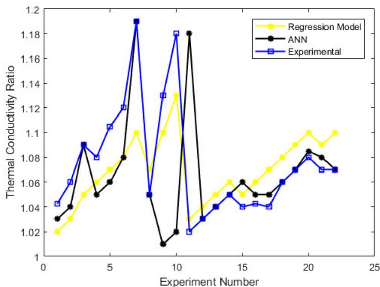
Fig. 3. Experimental vs. predicted values of thermal conductivity ratio
