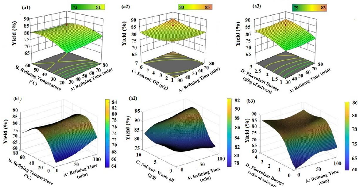
Fig. 5. The combined effect of refining time and refining temperature with (a1) CCD model (b1) ANN model; combined effect of refining time and solvent to oil ratio with (a2) CCD model and (b2) ANN model; combined effect of refining time and flocculant dosage with (a3) CCD model and (b3) ANN Model
