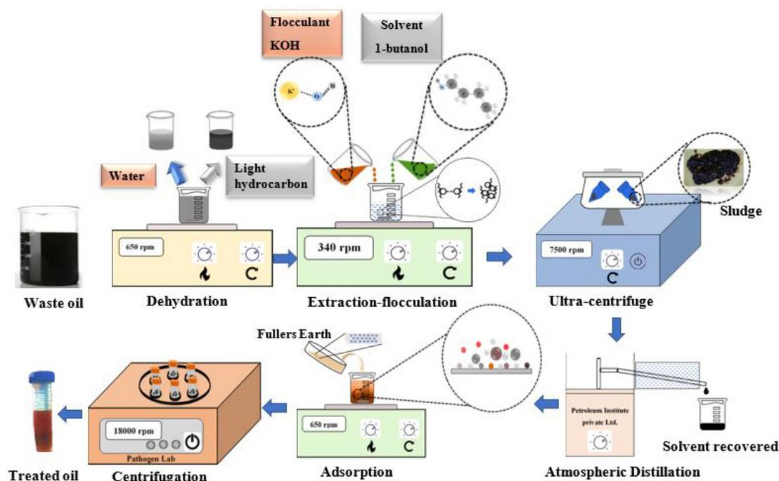
Fig. 1. Process flow diagram of extraction-flocculation process
