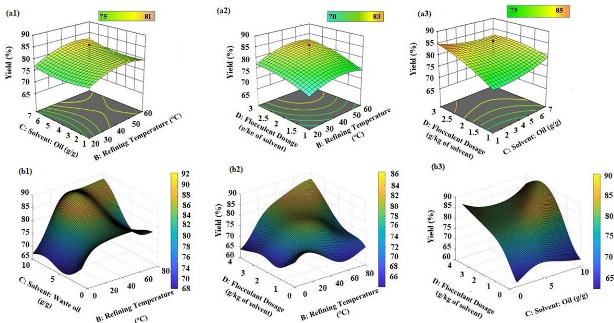
Fig. 6. The combined effect of refining temperature and solvent to waste oil ratio with (a1) CCD model (b1) ANN model; combined effect of refining temperature and flocculant dosage with (a2) CCD model (b2) ANN model; combined effect of solvent to waste oil ratio and flocculant dosage with (a3) CCD model (b3) ANN model
