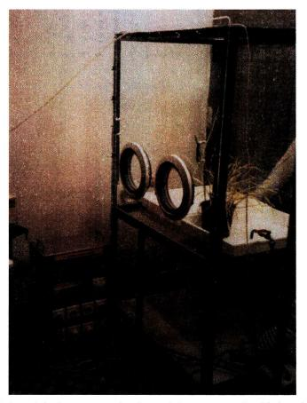
Fig. 2. General view of the  $O_3$  exposure chamber and the power supply with the relative humidity control unit
