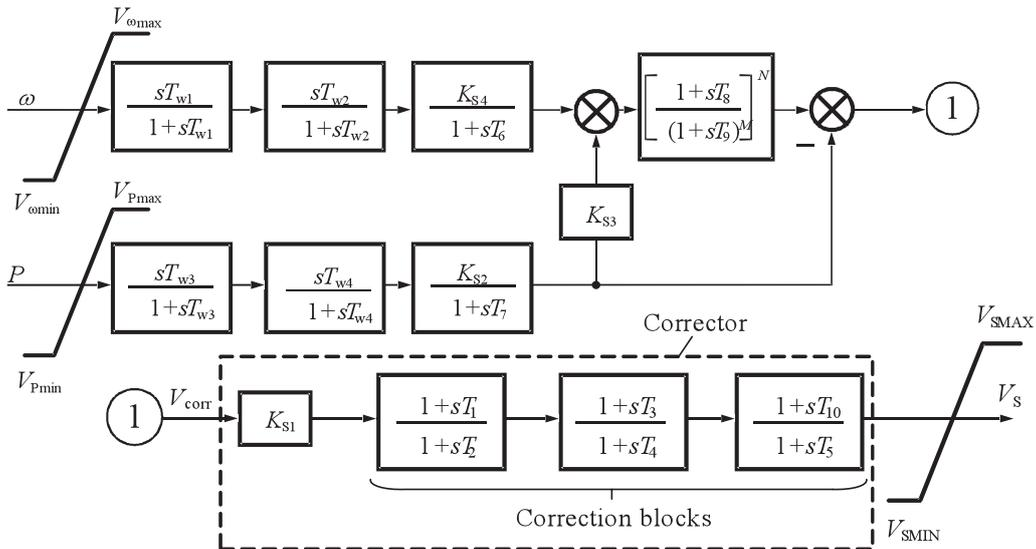
Fig. 1. Structural diagram of the dual input PSS2A stabiliser
