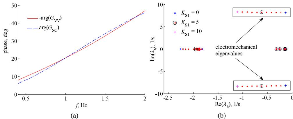
Fig. 5. Determination of the time constants of the PSS corrector by approximating the phase characteristics of the transfer function  $G_{VV}$  by the phase angle of the corrector  $G_{SC}$  (a); location of the eigenvalues of the system state matrix (rated load) when changing gain  $K_{S1}$ , selection of the value of gain  $K_{S1}$  (b)
