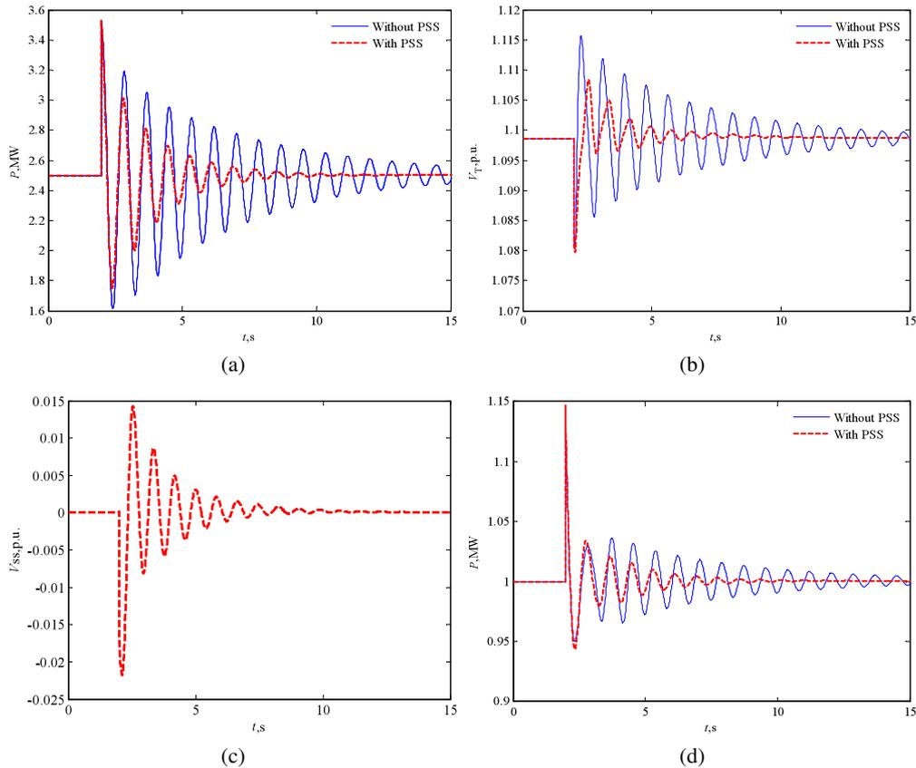
Fig. 8. The waveforms of instantaneous power (a); voltage (b); the PSS output signal (c) of the generator  $G_4$  as well as instantaneous power of the generator  $G_5$  (d)
