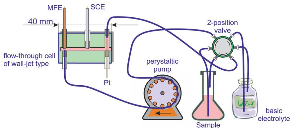
**Fig. 1.** A three-electrode measuring cell, consisting of a mercury film working electrode (MFE) based on glassy carbon, a saturated calomel reference electrode (SCE) and a platinum wire auxiliary electrode
