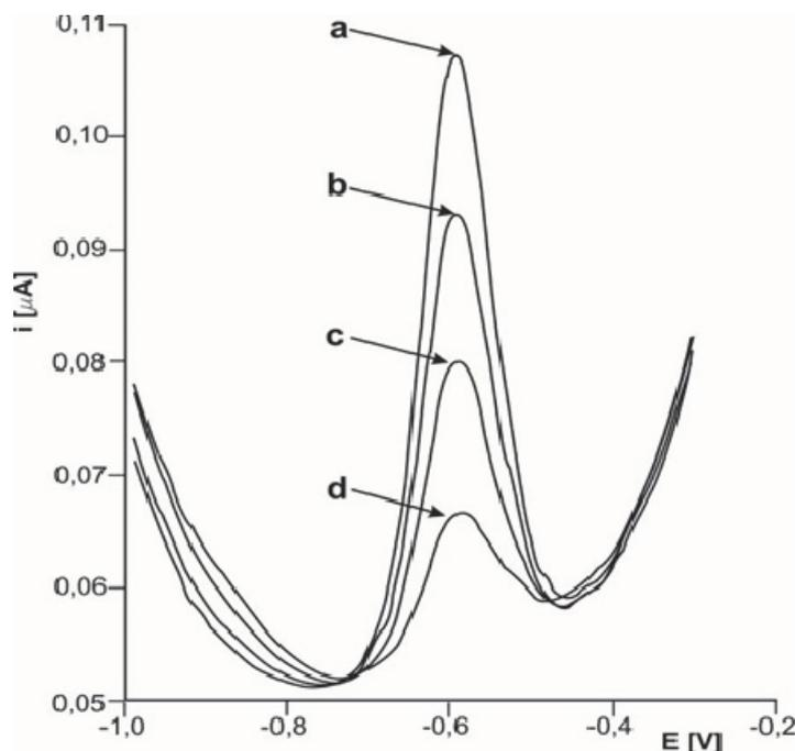
**Fig. 2.** Voltammograms of the sample (d) with sequential standard additions: 0.5 µg/L, 1 µg/L, 1.5 µg/L (respectively a,b,c) as well as the calibration graph. The base electrolyte 0.05 M EDTA (pH 4.5). Preconcentration potential -900mV vs. SCE; preconcentration time 600s, pulse amplitude 50 mV, step potential 2 mV.
