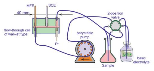
**Fig. 1.** A three-electrode measuring cell, consisting of a mercury film working electrode (MFE) based on glassy carbon, a saturated calomel reference electrode (SCE) and a platinum wire auxiliary electrode
