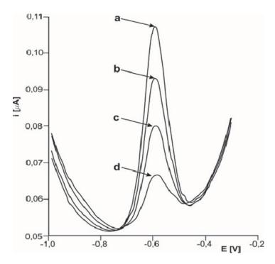
**Fig. 2.** Voltammograms of the sample (d) with sequential standard additions: 0.5 μg/L, 1 μg/L, 1,5 μg/L (respectively a,b,c) as well as the calibration graph. The base electrolyte 0.05 M EDTA (pH 4.5). Preconcentration potential -900mV vs. SCE; preconcentration time 600s, pulse amplitude 50 mV, step potential 2 mV.
