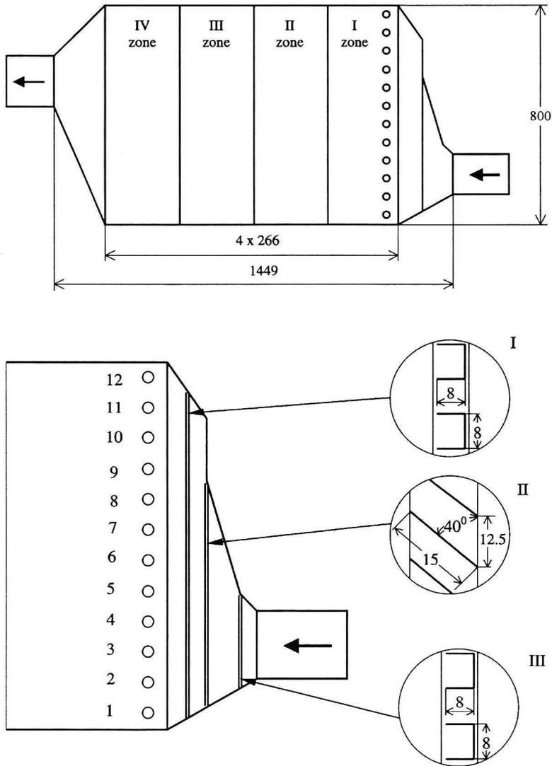
Fig. 2. Model of a horizontal electrostatic precipitator: (a) diagram showing the horizontal electrostatic precipitator (in millimetres), (b) diagram showing the location of shaping and moderating elements in the diffuser; I – distribution screen (consisting of horizontal C-profiles) coefficient of perforation 55%, II – guide vanes, III - distribution screen (consisting of horizontal C-profiles) coefficient of perforation 37%
