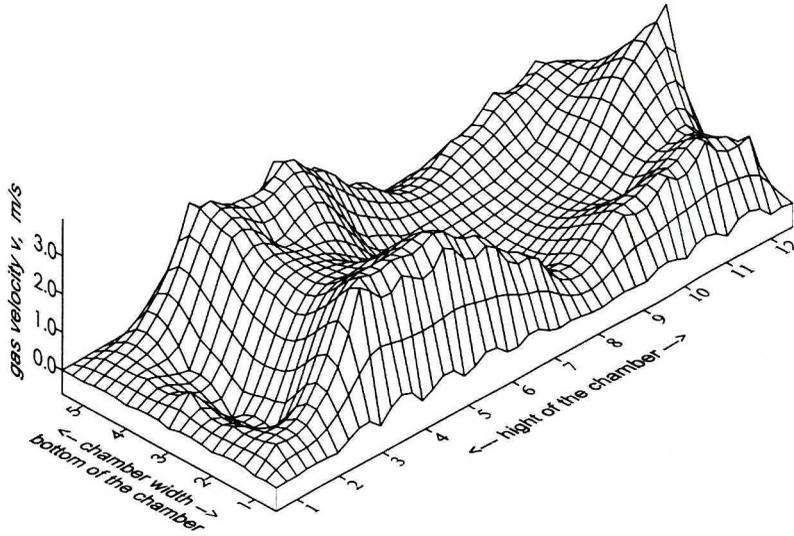
Fig. 3. Velocity distribution at the inlet of the chamber of the electrostatic precipitator for a concave profile
