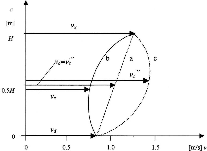
Fig. 1. Examples of velocity profiles of flue gas in the vertical cross section of the chamber of an electrostatic precipitator where the flow is dominant in the upper part of the chamber: a – linear profile, b – concave profile, c – convex profile
