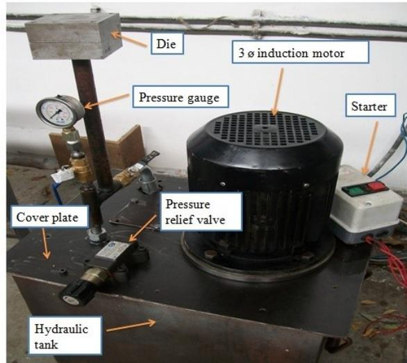
Fig. 2. Sheet hydro-mechanical drawing set-up
