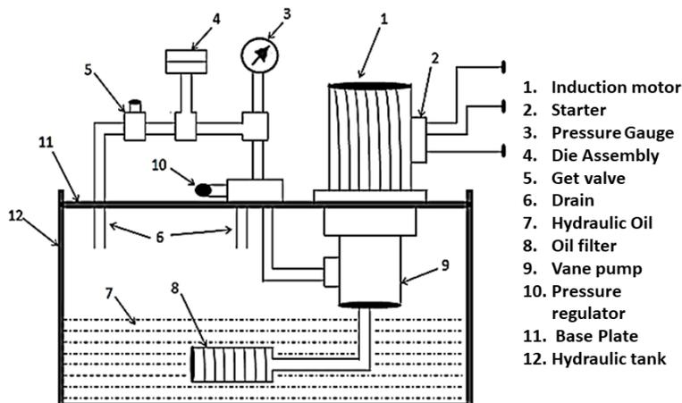
Fig. 1. Schematic of sheet hydro-mechanical drawing set-up
