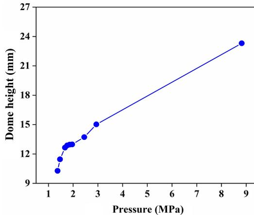
Fig. 4. Effect of hydraulic pressure on the dome height of deformed aluminium 8011 alloy sheet
