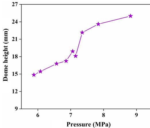
Fig. 6. Effect of hydraulic pressure on the dome height of deformed copper 12200 alloy sheet
