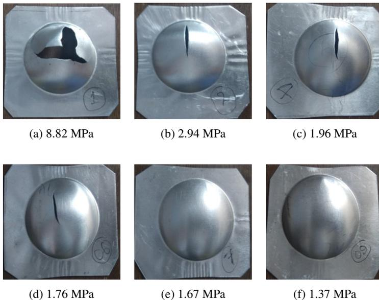
Fig. 5. Deformed aluminium 8011 alloy sheet under different hydraulic pressure
