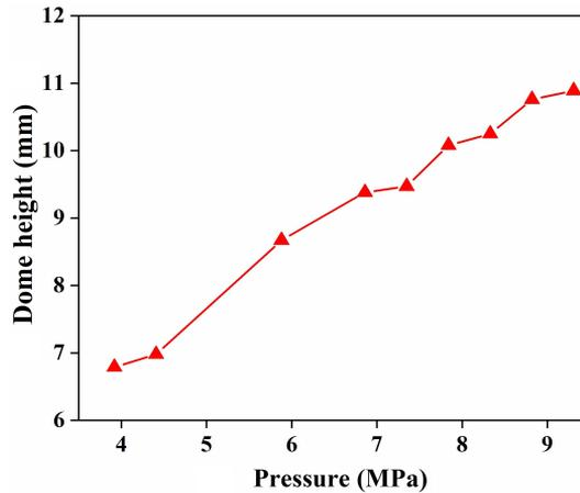
Fig. 8. Effect of hydraulic pressure on the dome height of deformed steel EN10130 alloy sheet
