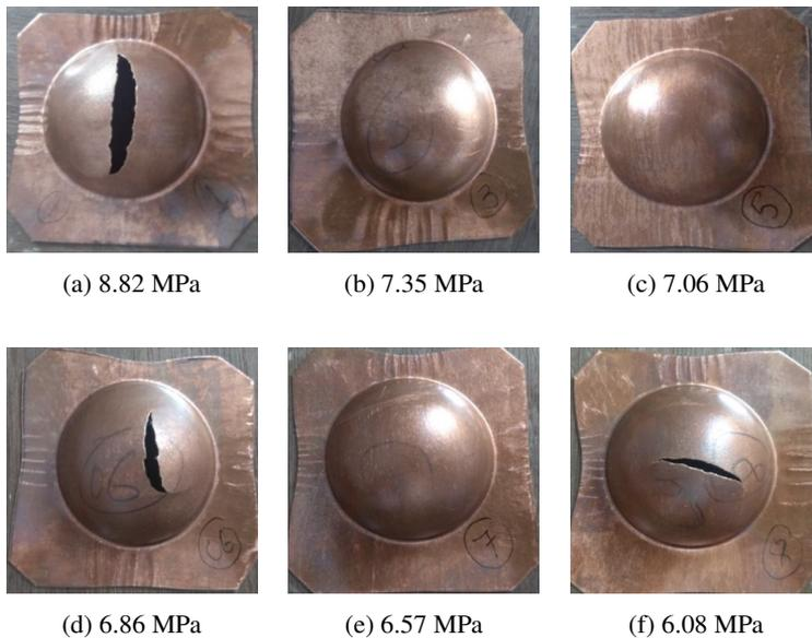
Fig. 7. Deformed copper C12200 alloy sheet under different hydraulic pressure
