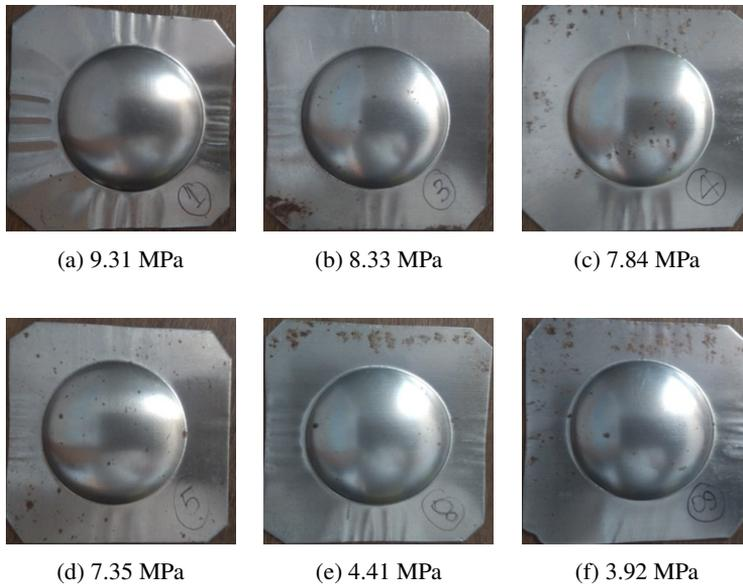
Fig. 9. Deformed steel EN10130 alloy sheet under different hydraulic pressure
