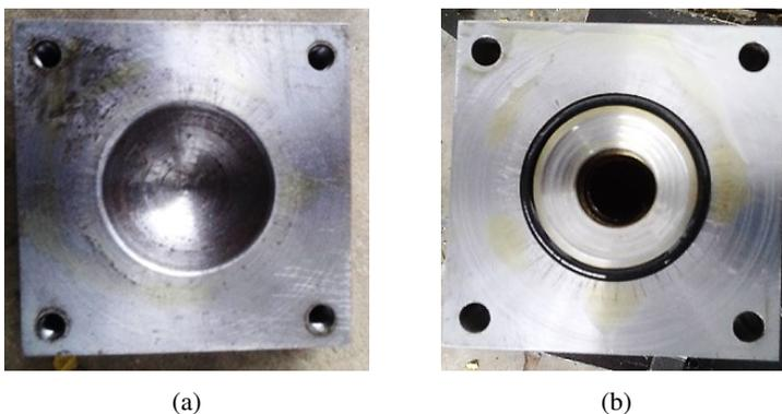
Fig. 3. Hemispherical die (a) and oil seal attached blank holder (b)
