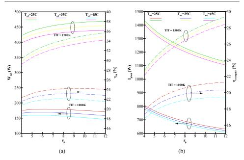
Fig. 6. Variation of  $W_{\text{net}}$ , and  $\eta_{\text{th}}$  (a) and  $I_{\text{plant}}$  and  $\eta_{\text{exergetic}}$  (b) of ABC cycle w.r.t.  $r_p$ , *TIT*, and  $T_{\text{ref}}$  of set 3
