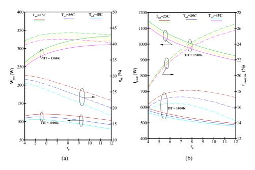
Fig. 4. Variation of  $W_{\text{net}}$ , and  $\eta_{\text{th}}$  (a) and  $I_{\text{plant}}$  and  $\eta_{\text{exergetic}}$  (b) of ABC cycle w.r.t.  $r_p$ , *TIT*, and  $T_{\text{ref}}$  of set 2
