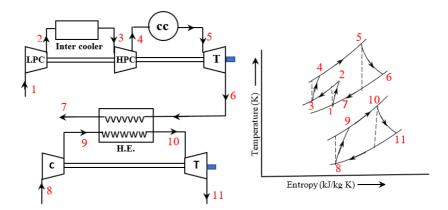
Fig. 5. Schematic and T-s diagram of set 3
