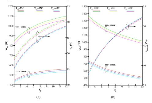
Fig. 8. Variation of  $W_{\text{net}}$ , and  $\eta_{\text{th}}$  (a) and  $I_{\text{plant}}$  and  $\eta_{\text{exergetic}}$  (b) of ABC cycle w.r.t.  $r_p$ , *TIT*, and  $T_{\text{ref}}$  of set 4
