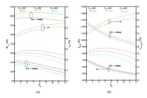
Fig. 2. Variation of  $W_{\text{net}}$ , and  $\eta_{\text{th}}$  (a) and  $I_{\text{plant}}$  and  $\eta_{\text{exergetic}}$  (b) of ABC cycle w.r.t.  $r_p$ , *TIT*, and  $T_{\text{ref}}$  of set 1
