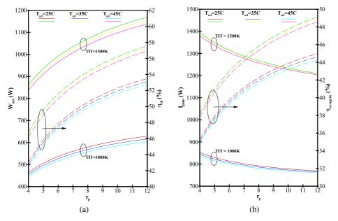
Fig. 10. Variation of  $W_{\text{net}}$ , and  $\eta_{\text{th}}$  (a) and  $I_{\text{plant}}$  and  $\eta_{\text{exergetic}}$  (b) of ABC cycle w.r.t.  $r_p$ , *TIT*, and  $T_{\text{ref}}$  of set 5
