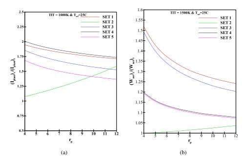
Fig. 12. Variation of the ratio of total exergy destruction of the ABC to its topping cycle at TIT = 1000 K (a), and TIT = 1500 K (b)
