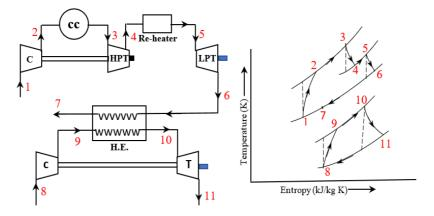
Fig. 7. Schematic and T-s diagram of set 4
