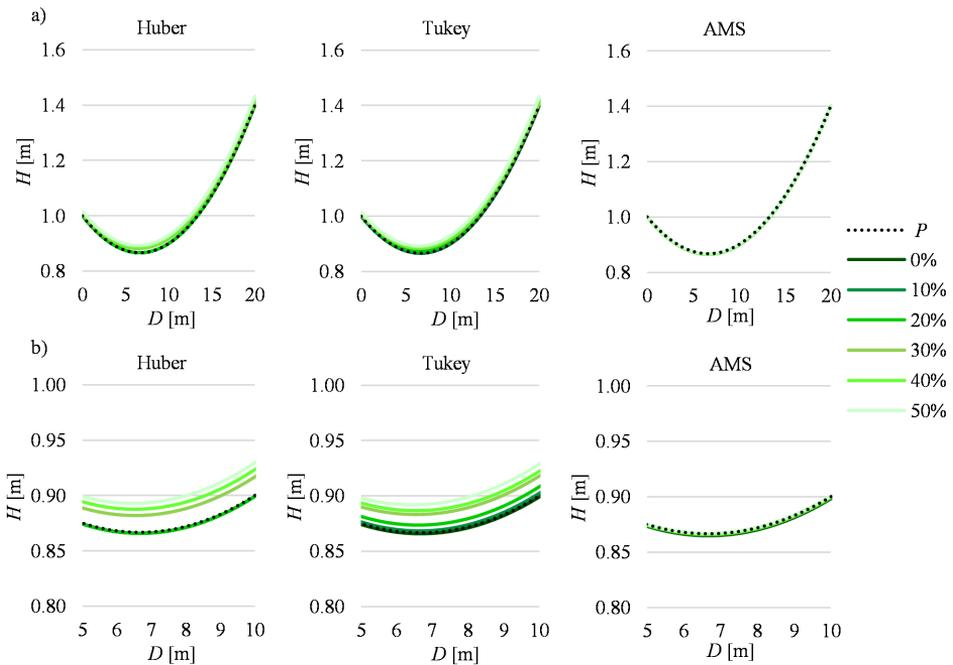
Fig. 4. Estimated terrain profiles for the Huber, Tukey, and AMS estimates for different percentages of outliers: for the interval from 0 to 20 m, for the interval from 5 to 10 m ( $P$  is the simulated terrain profile)
