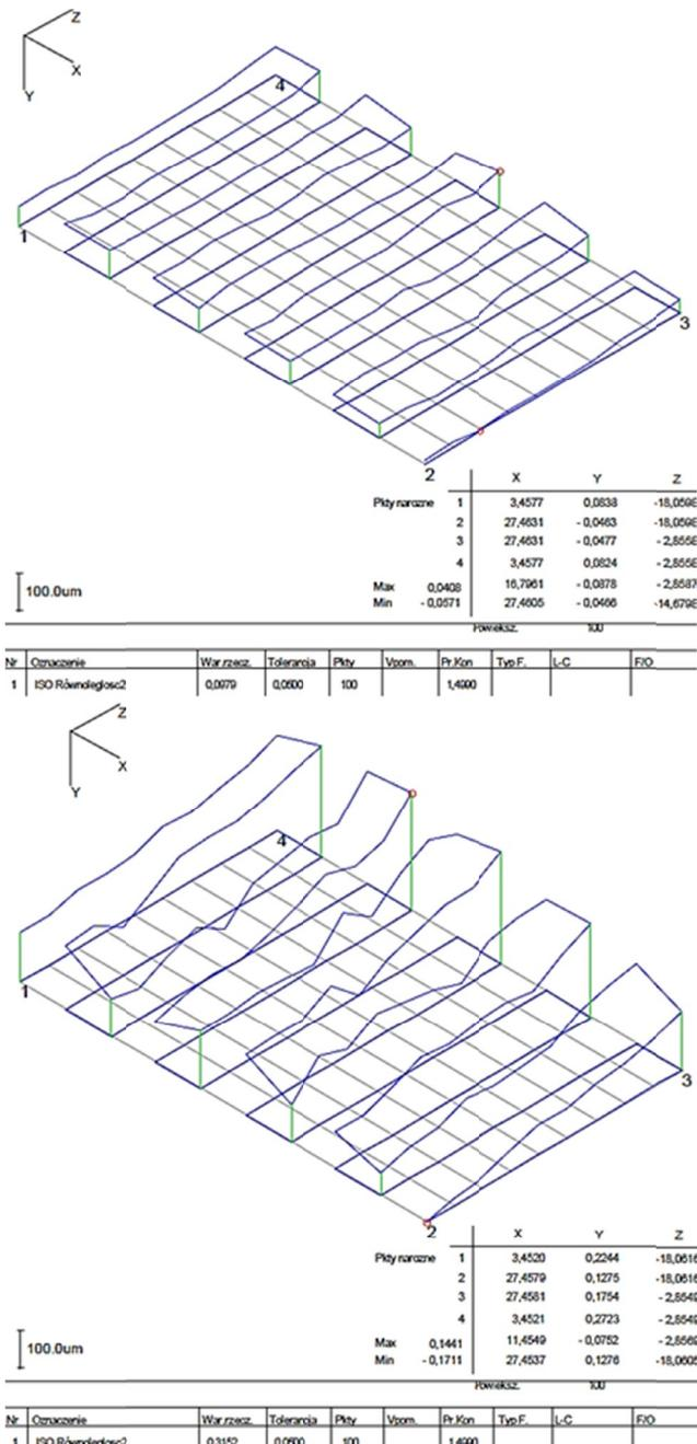
Fig. 11. Parallelism for St10S1 (top) and St10S10 (bottom)
