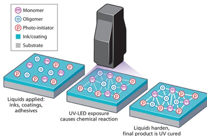
Fig. 1. Polymerization of resin in UV curing [2]
