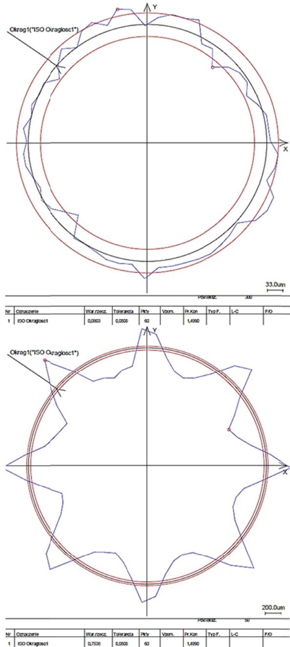
Fig. 12. Roundness for St10S1 (top) St10S10 (bottom)
