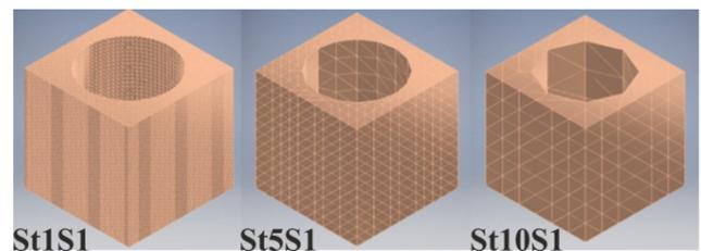
Fig. 7. The view of the meshes with constant sag value and different step
