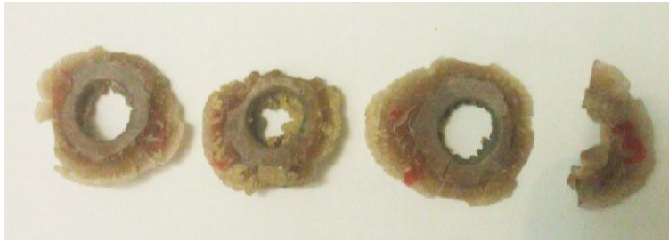
Fig. 14. The local plugging mechanism occurring in the nano-composite targets Al-No-T-3 under the cylindrical projectiles' impact
