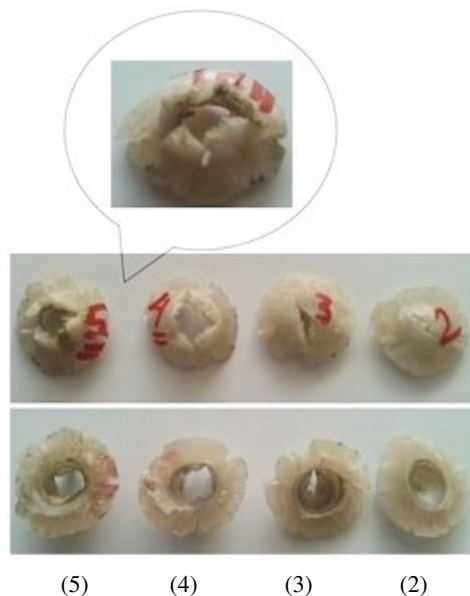
Fig. 12. Changing the failure mechanism resulted from velocity's rise of conical projectiles in the front and rear of the separated parts (plugs) of specimen Al-T-3 from dishing (no. 2) to petalling (no. 4 and 5)
