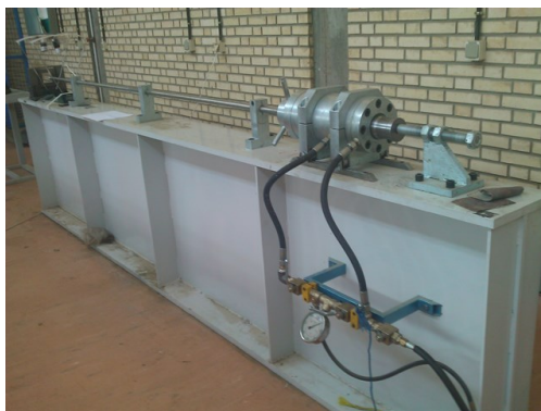
Fig. 1. Gas gun used for performing ballistic tests
