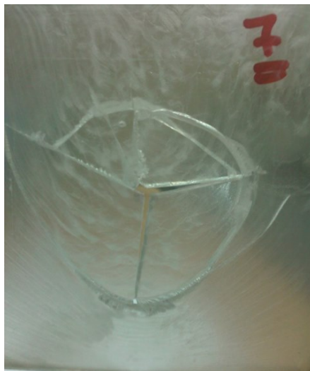
Fig. 5. The broken neat polycarbonate target after the hemispherical projectile impact with an incident velocity under the ballistic limit velocity
