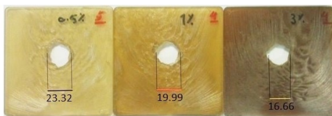
Fig. 15. The reduction of perforations' diameter produced in the nano-composite targets contained untreated nano particles by increasing the weight percentage of nano contents (from left to right of illustration; dimensions are in millimeter)
