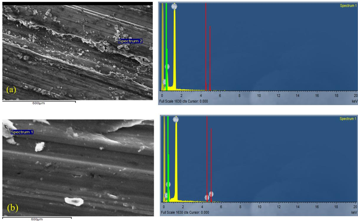
Fig. 10. EDS graphs of worn out a) pure Mg sample and b) TiC reinforced composite
