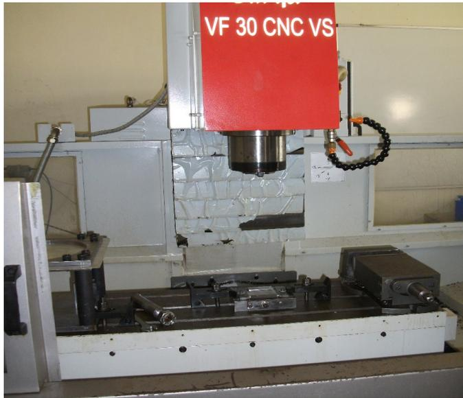
Fig. 1. Actual set-up on CNC vertical milling machine
