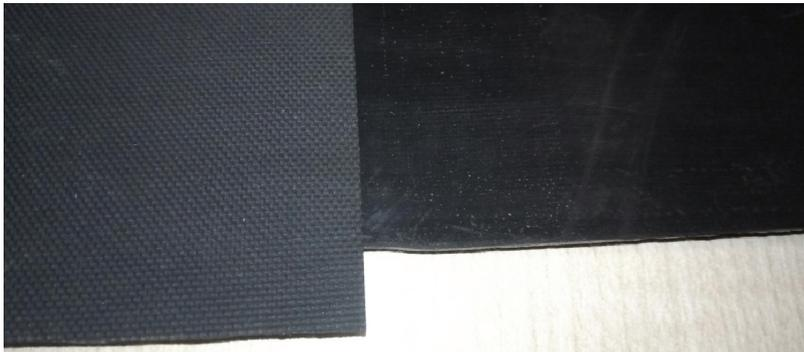
Fig. 2. Two types (outside and inside) EPDM membranes – visible different surface textures on the backside
