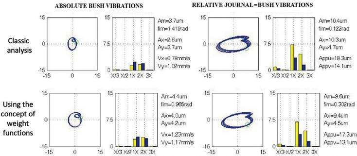
Calculation results for unstable working conditions caused by the cracked generator rotor
