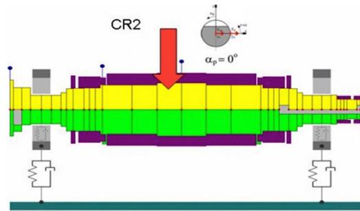
Simulation of the rotor crack located in the middle part of the generator.
