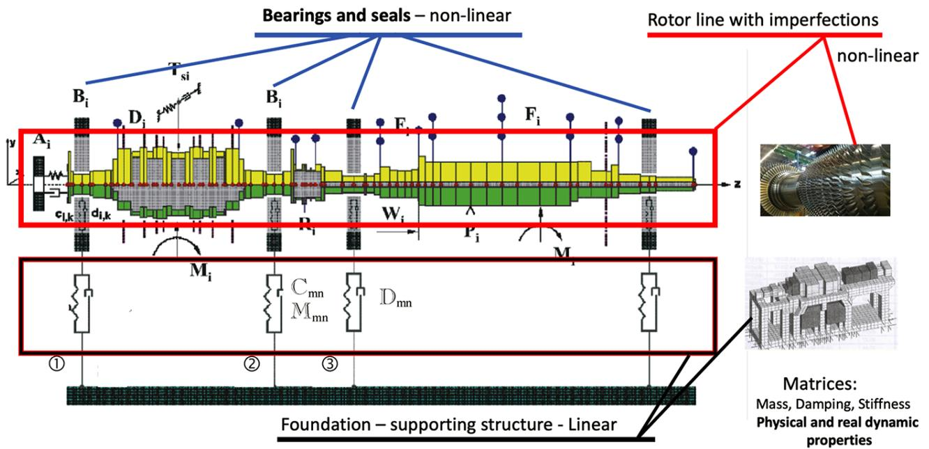
Fig. 1. Main subsystems of the turbomachine and the main questions arising from the attempt to describe them mathematically and accurately
