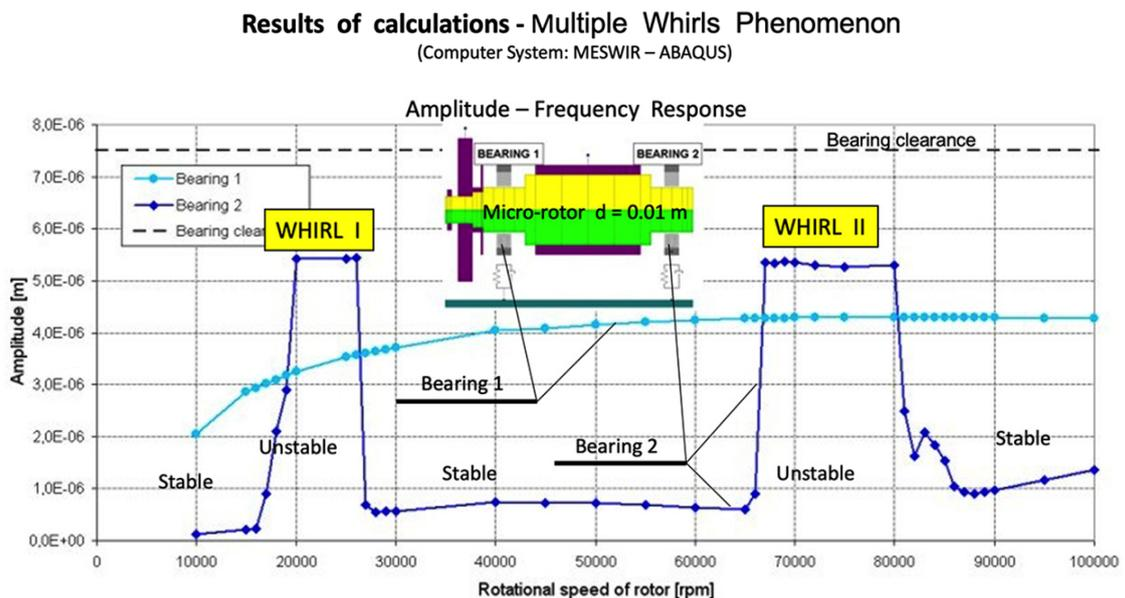
Fig. 12. Computer simulation results illustrating the occurrence of multiple whirls
