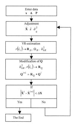
Fig. 2. The general scheme of iterative adjustment
