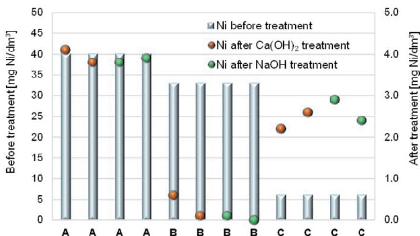
Fig. 2. The content of nickel ions before and after the neutralization process with the use of either calcium hydroxide or sodium hydroxide for model wastewater:
