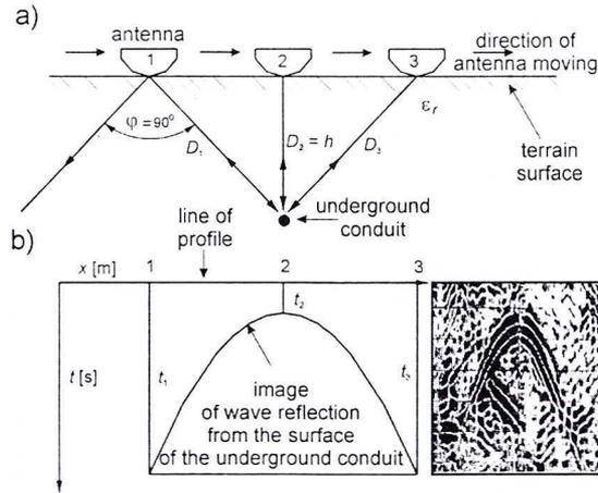
Fig. 2. Overall diagram of construction of the echogram of underground installations for measurements with the use of the geo-radar method
