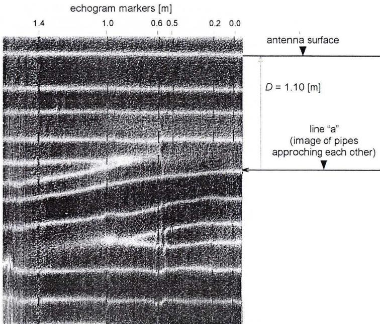
Fig. 5. Echogram from measurements of the horizontal resolution of two steel pipes
