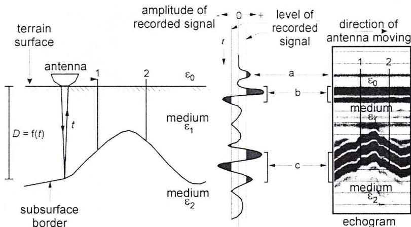
Fig. 1. Overall diagram of measurements using the geo-radar method; *a* – initial impulse, *b* – impulse reflected from the Earth surface, *c* – impulse reflected from the subsurface border,  $D = f(t)$  – depth as the function of time,  $\epsilon_1, \epsilon_2$  – dielectric constants of media
