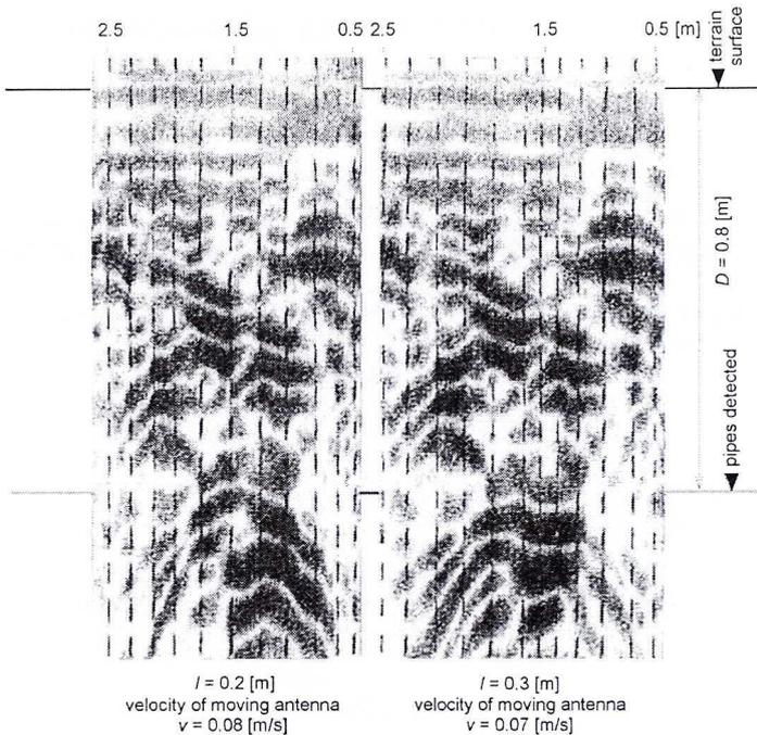
Fig. 7. Echograms of two steel pipes obtained using the 200 MHz antenna in the medium of the dielectric constant  $\epsilon_r = 19$
