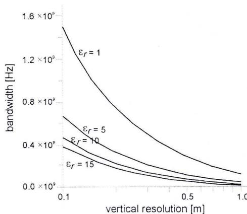
Fig. 4. Relations between the vertical resolution and the antenna bandwidth for various dielectric constants  $\epsilon_r$
