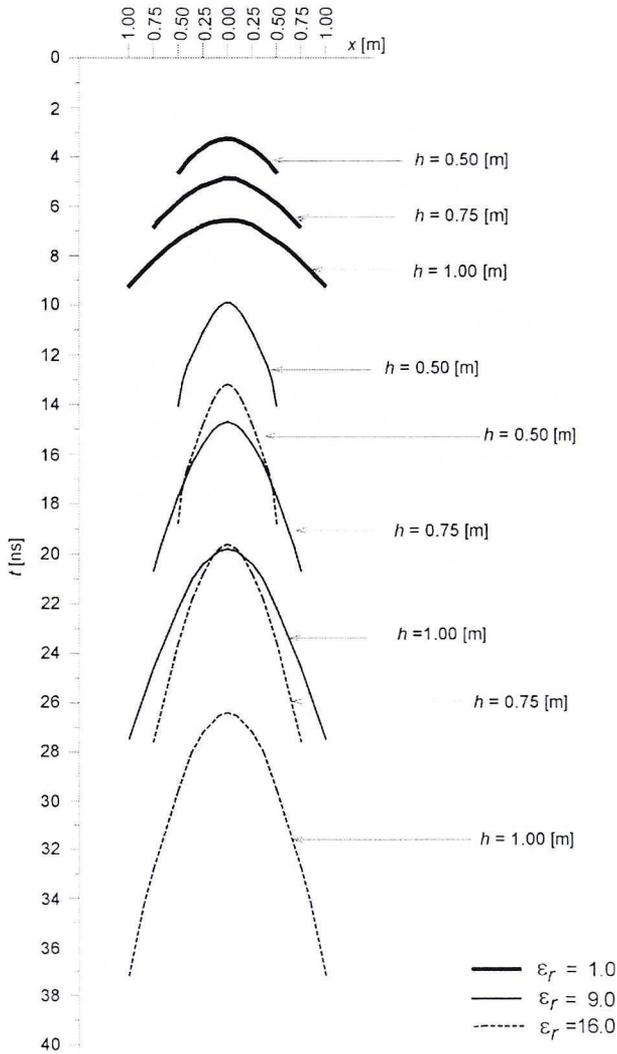
Fig. 3. Model of echograms of a linear object of circular cross-section for various values of the dielectric constant  $\epsilon_r$  and various depths  $h$
