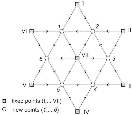
Rys. 17. The test network of geometrical levelling
