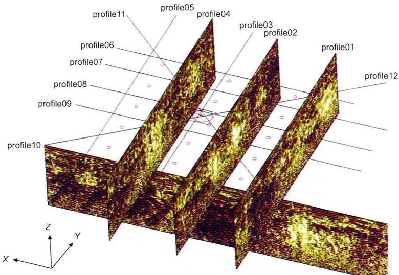
Fig. 4. Correlation of structures on radargram cross-sections
