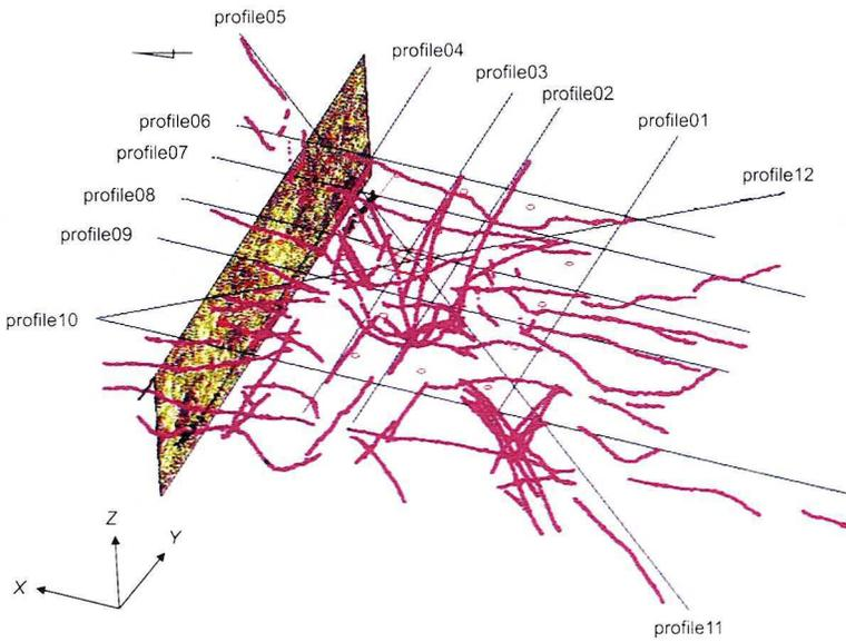
Fig. 3. The spatial model of a sinkhole created from radar data with the AutoCAD program
