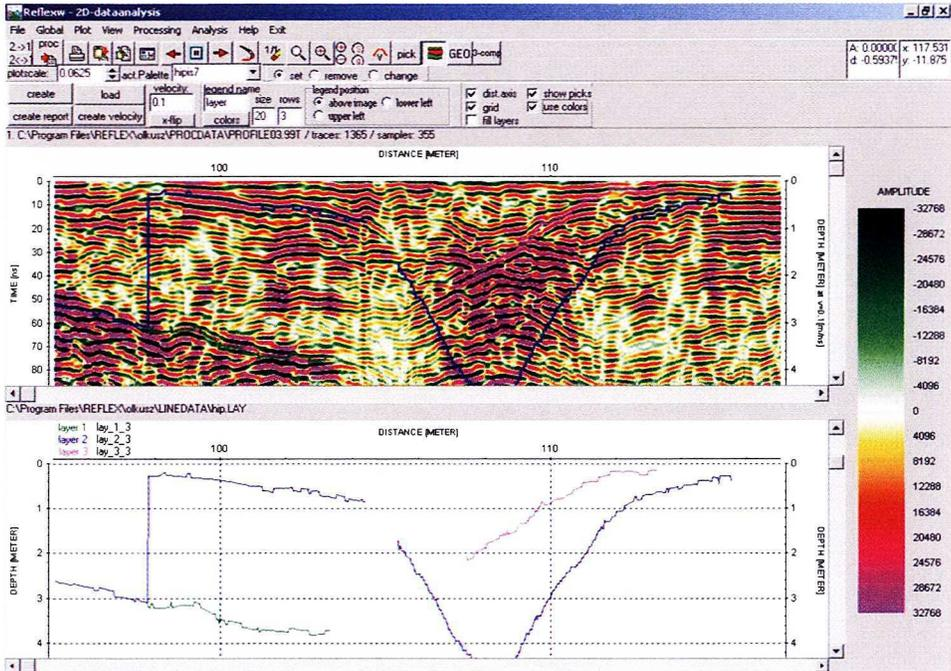
Fig. 2. An example of vectorization on a radargram using the ReflexW software
