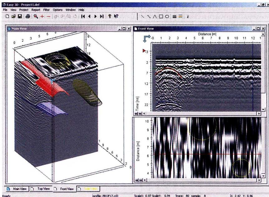
Fig. 1. The three-dimensional radar model created with the Easy 3D program
