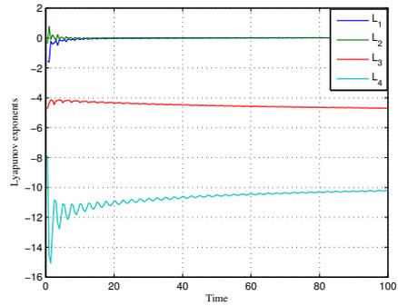
(b) The Lyapunov exponent for Modified Colpitts oscillator with  $\varepsilon_1 = 1, \varepsilon_2 = 20, \sigma_1 = 1.49, \sigma_2 = 0.872, \alpha = 255/256, \gamma = 25.80$  with initial condition  $(x_1, x_2, x_3, x_4) = (1, 1, 1, 1)$
