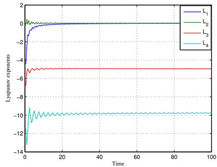
(d) The Lyapunov exponent for Modified Colpitts oscillator with  $\varepsilon_1 = 1, \varepsilon_2 = 20, \sigma_1 = 1.49, \sigma_2 = 0.872, \alpha = 255/256, \gamma = 25.80$  with initial condition  $(x_1, x_2, x_3, x_4) = (0.0001, 0.0001, 0.0001, 0.0001)$
