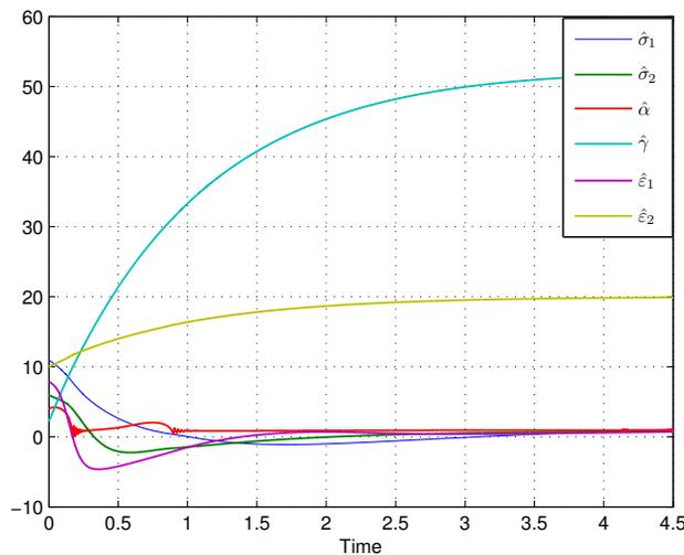
Figure 4: The parameter estimation of the modified Colpitts oscillator
