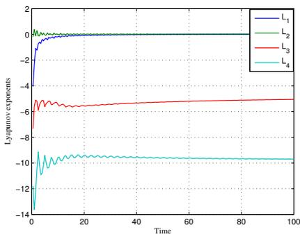
(e) The Lyapunov exponent for Modified Colpitts oscillator with  $\varepsilon_1 = 1, \varepsilon_2 = 20, \sigma_1 = 1.49, \sigma_2 = 0.872, \alpha = 255/256, \gamma = 25.80$  with initial condition  $(x_1, x_2, x_3, x_4) = (0.00001, 0.00001, 0.00001, 0.00001)$
