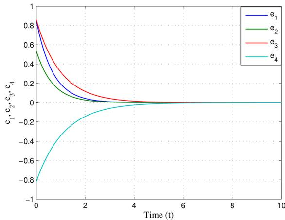
Figure 7: Error Dynamics of Chaotic Colspitts oscillator
