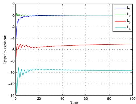
(f) The Lyapunov exponent for Modified Colpitts oscillator with  $\varepsilon_1 = 1, \varepsilon_2 = 20, \sigma_1 = 1.49, \sigma_2 = 0.872, \alpha = 255/256.5, \gamma = 25.80$  with initial condition  $(x_1, x_2, x_3, x_4) = (0.0001, 0.0001, 0.0001, 0.0001)$
