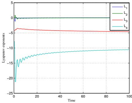
(a) The Lyapunov exponent for Modified Colpitts oscillator with  $\varepsilon_1 = 1, \varepsilon_2 = 20, \sigma_1 = 1.49, \sigma_2 = 0.872, \alpha = 255/256, \gamma = 25.80$  with initial condition  $(x_1, x_2, x_3, x_4) = (2.6758, 0.7834, 8.2345, 1.4387)$
