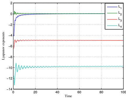
(c) The Lyapunov exponent for Modified Colpitts oscillator with  $\varepsilon_1 = 1, \varepsilon_2 = 20, \sigma_1 = 1.49, \sigma_2 = 0.872, \alpha = 255/256, \gamma = 25.80$  with initial condition  $(x_1, x_2, x_3, x_4) = (0.001, 0.001, 0.001, 0.001)$
