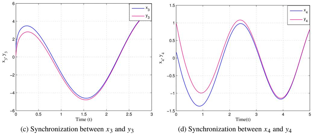
Figure 6: Synchronization of the Modified Colpitts oscillator
