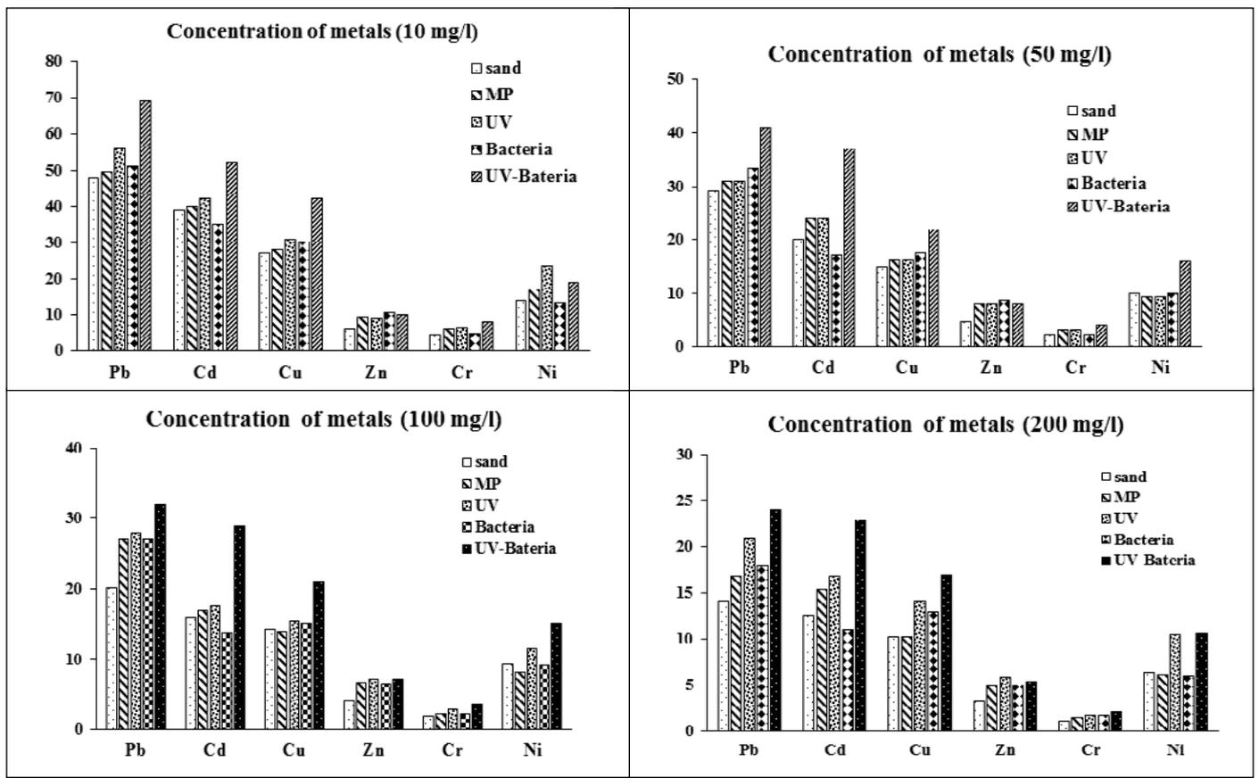
Fig. 4. Percentage of adsorption of heavy metals on various compounds of sand and micro-plastics, under UV irradiation and bacterial culture at concentrations of 10, 50, 100 and 200 mg/l
