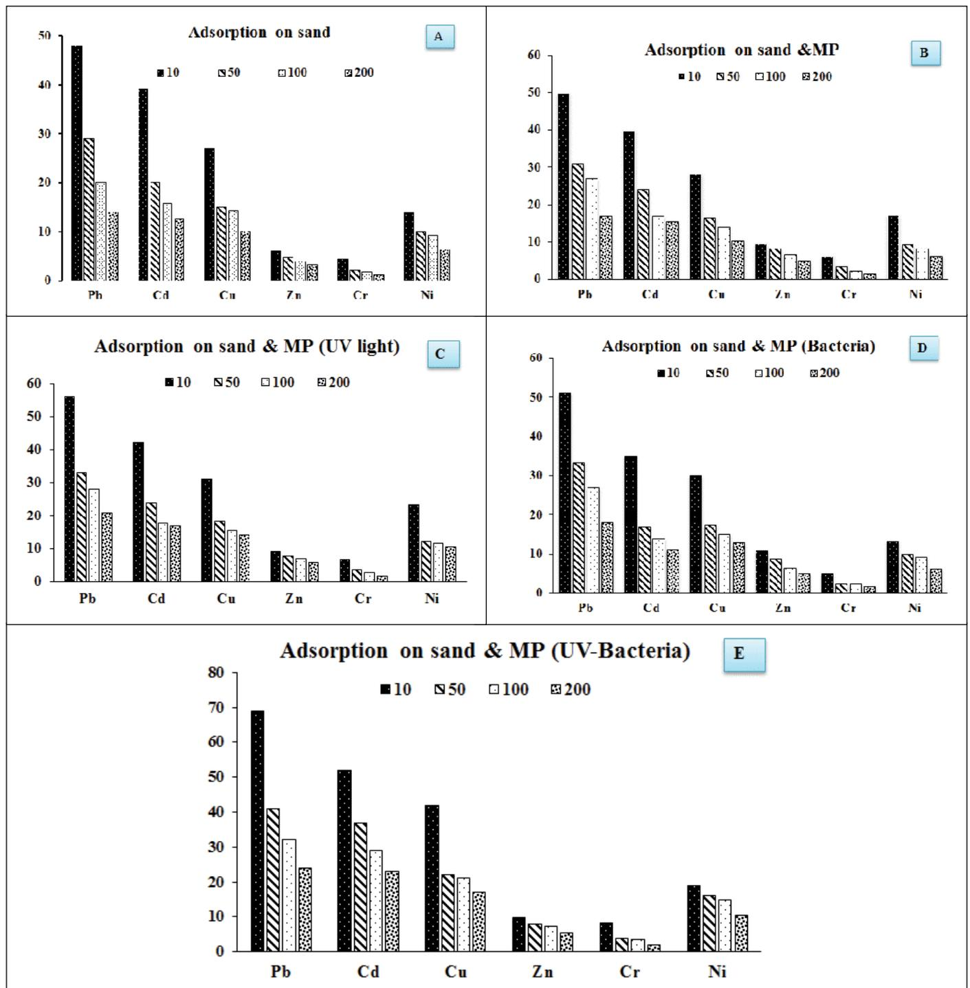
**Fig. 3.** Adsorption of heavy metals on A) Sand, B) Sand and micro-plastics C) Sand and micro-plastics exposed to UV D) Sand and micro-plastics containing bacteria E) Sand and micro-plastics containing bacteria exposed to UV
