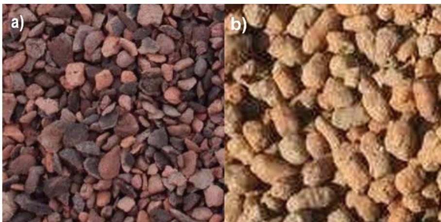
Fig. 2. Lightweight aggregate used in the tested concrete mixes: a) sintered fly ash, b) thermally expanded silty clay
