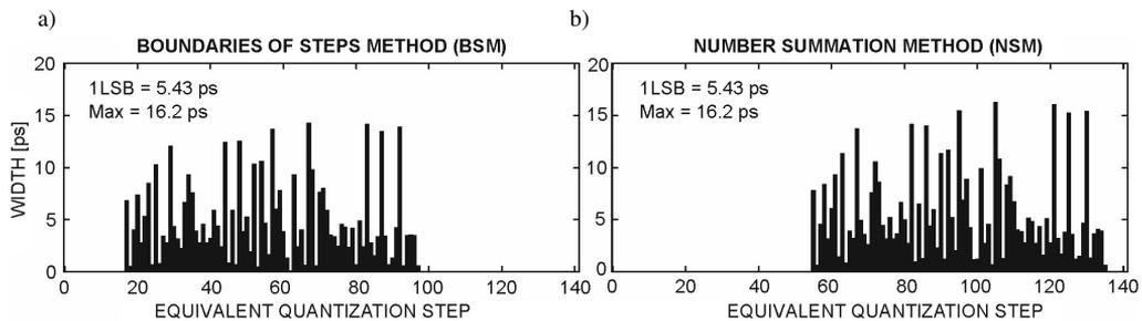
Fig. 7. Widths of ECL quantization steps determined by the two tested methods: boundaries of steps (a) and number summation (b).
