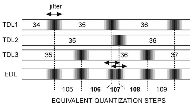
Fig. 10. Illustration of the influence of timing jitter phenomenon of the boundaries of quantization steps on equivalent quantization steps widths.
