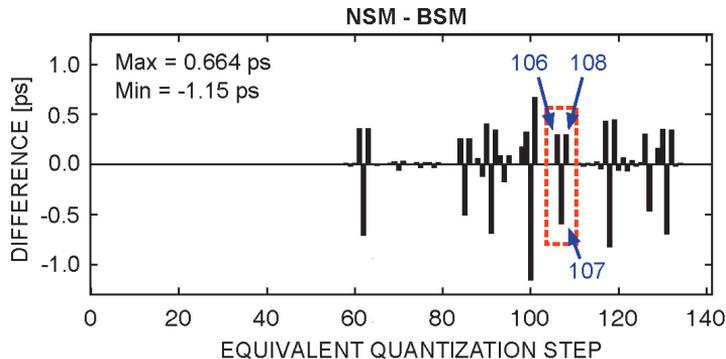
Fig. 8. Differences in the widths of equivalent quantization steps determined in both studied methods.
