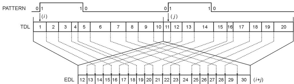
Fig. 4. Method of creating equivalent quantization steps for the converter with multiedge signal.
