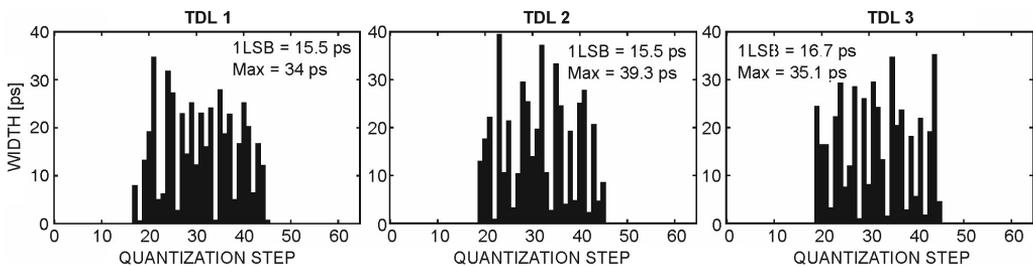
Fig. 6. Widths of the quantization steps for three time coding delay lines of a T/D converter.
