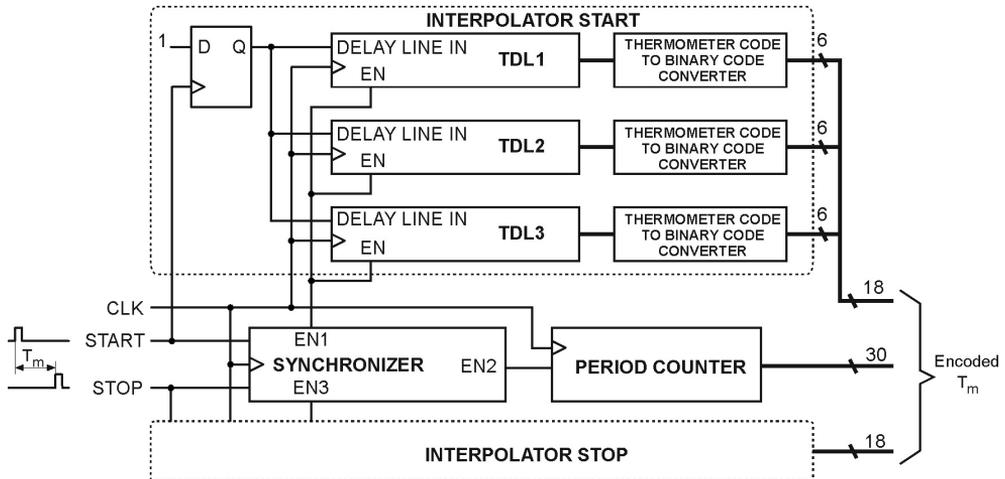
Fig. 5. Simplified block diagram of the interpolation time counter.
