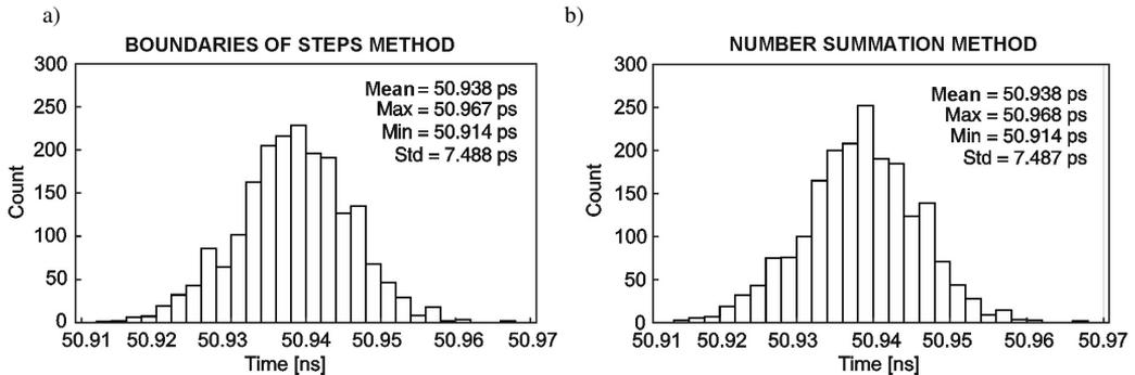
Fig. 9. Distributions of measurement results of an exemplary time interval obtained by means of equivalent transfer functions determined using the methods based consecutively on: evaluation of the quantization steps boundaries (a) and summation of quantization steps indexes (b).
