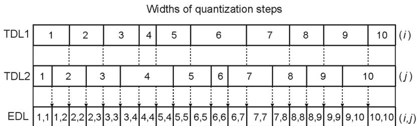
Fig. 2. Method for creating equivalent quantization steps for two independent time coding delay lines.
