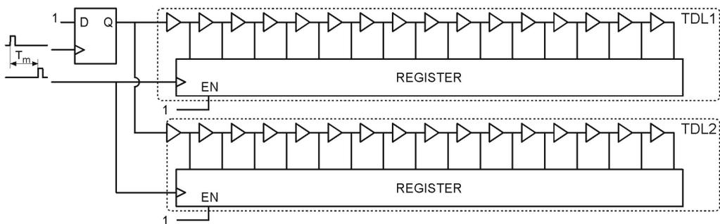
Fig. 1. Time-to-digital converter with two independent time coding delay lines.
