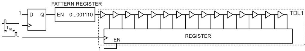
Fig. 3. T/D converter based on multiedge signal propagation in a single time coding delay line.
