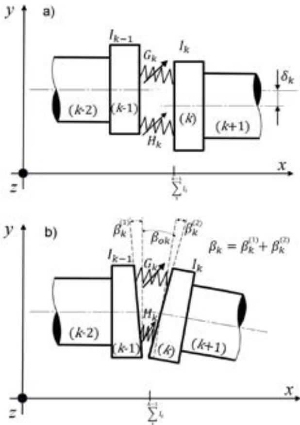
**Fig.2.** The model of the coupling with an inner anisotropy and parallel (a) and angular (b) misalignment
