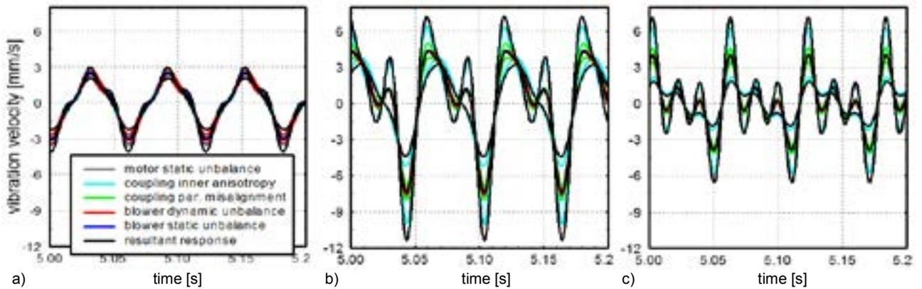
Fig.9. Vibration velocity fluctuations at housings of bearing #1 (a), #3 (b) and #4 (c) induced by system imperfections
