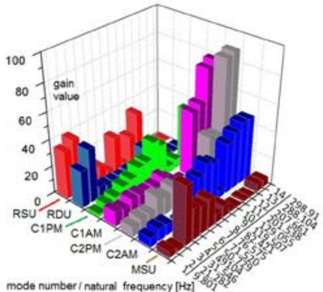
Fig.7. External excitation gains for successive eigenmodes of the blower rotor-shaft system
