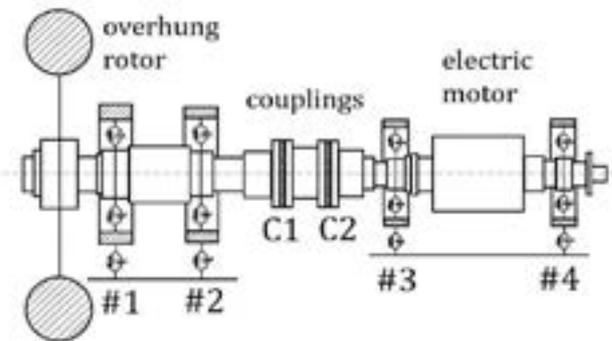
**Fig.3.** The industrial blower with an overhung rotor: the real object and its hybrid mechanical model
