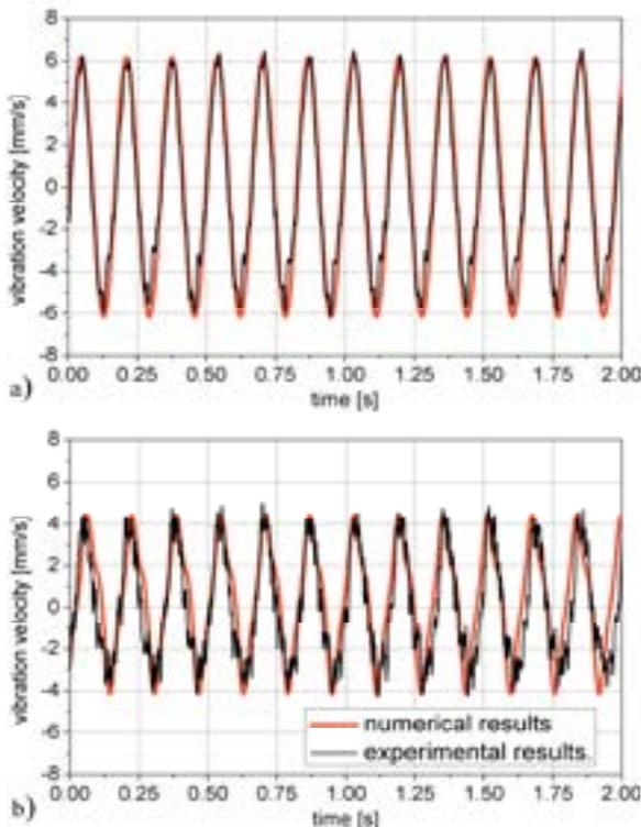
**Fig.4.** Measured and calculated vibration velocities at housings of bearing #1 (a) and bearing #3 (b)
