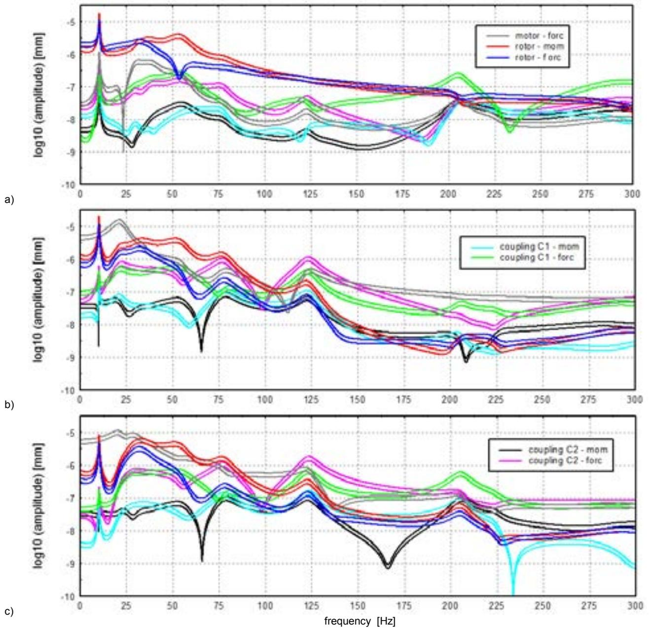
Fig.8. Interval frequency response characteristics at housings of bearing #1 (a), #3 (b) and #4 (c) induced by system imperfections
